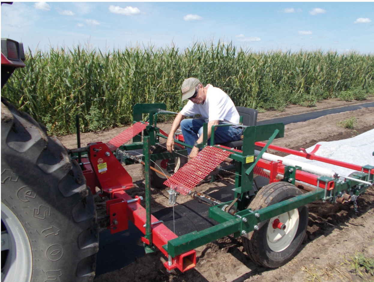
Figure 1. Tractor mounted tunnel layer implement inserting wire hoops and establishing row cover over hoops. The process is semi-mechanized requiring an operator to singulate and place the wire for hoops into the insertion mechanism.
