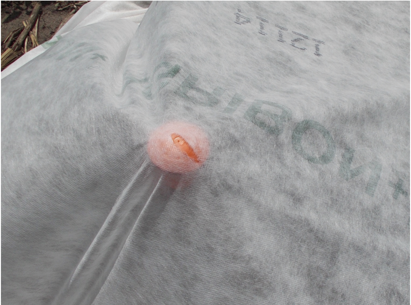
Figure 5. Plastic end cap atop support abrading through spunbond polypropylene cover material.
