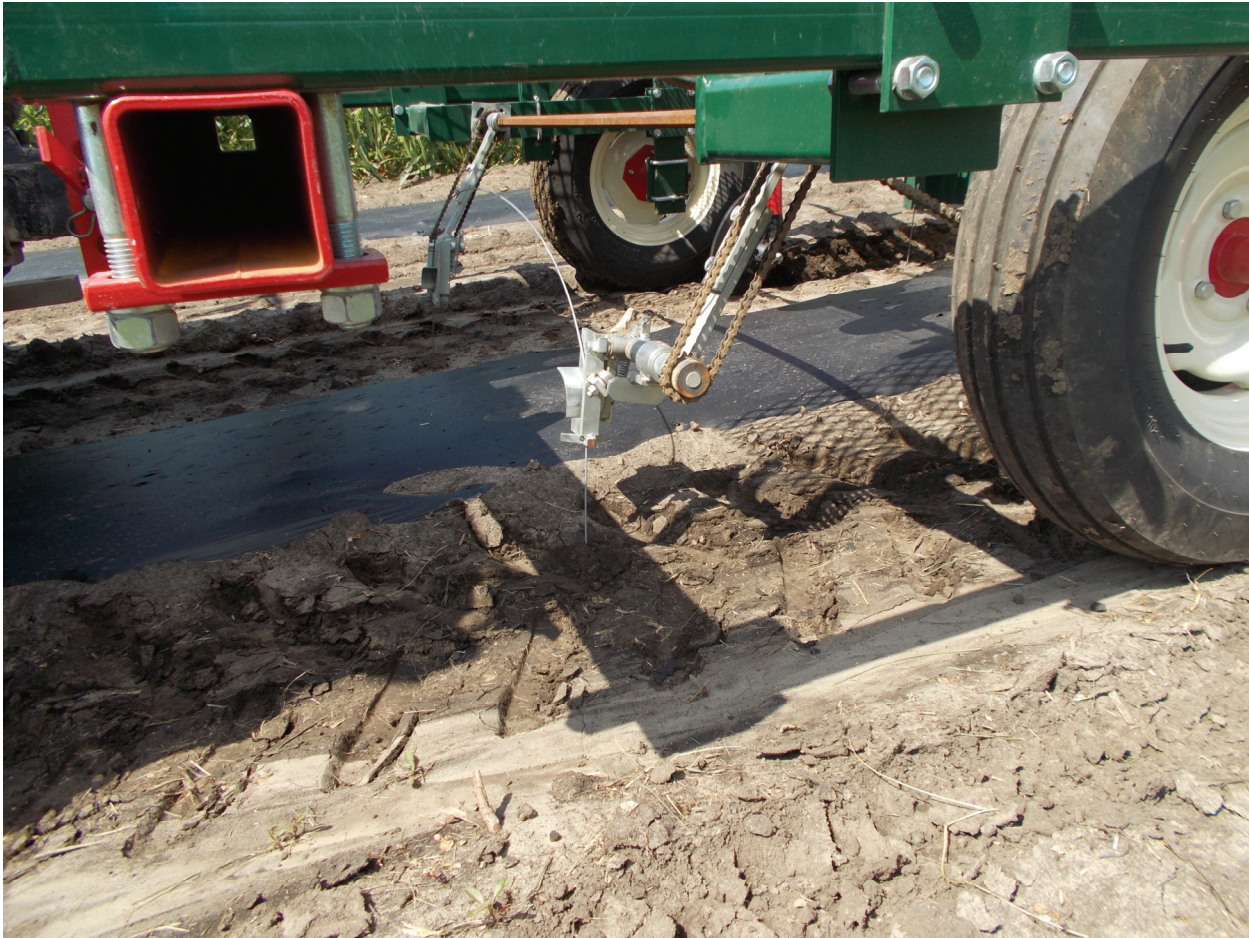
Figure 2. Wire inserted by cam-activated fingers on two rotating arms.
