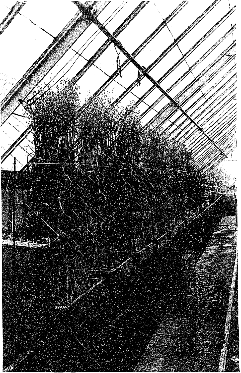
Figure 4. High voltage experiment with oats, 1931; includes six treated lots and two controls. Treated lots received currents at 7,000 to 20,000 volts for a 10 to 15 minute period daily. On this date, May 12, the controls are in the second and sixth locations, counting from the near end.
