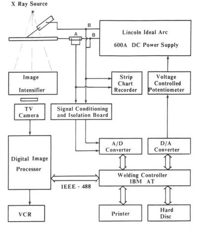
Fig. 2 Schematic diagram of experimental arrangement for intelligent process control of weld.
