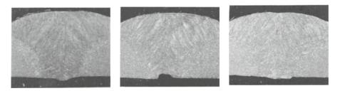
Fig. 5 Top row: Brightness profiles of images with computer decision: Complete (left and right) and incomplete (middle). Bottom row: Corresponding photographs of weld cross-sections.
