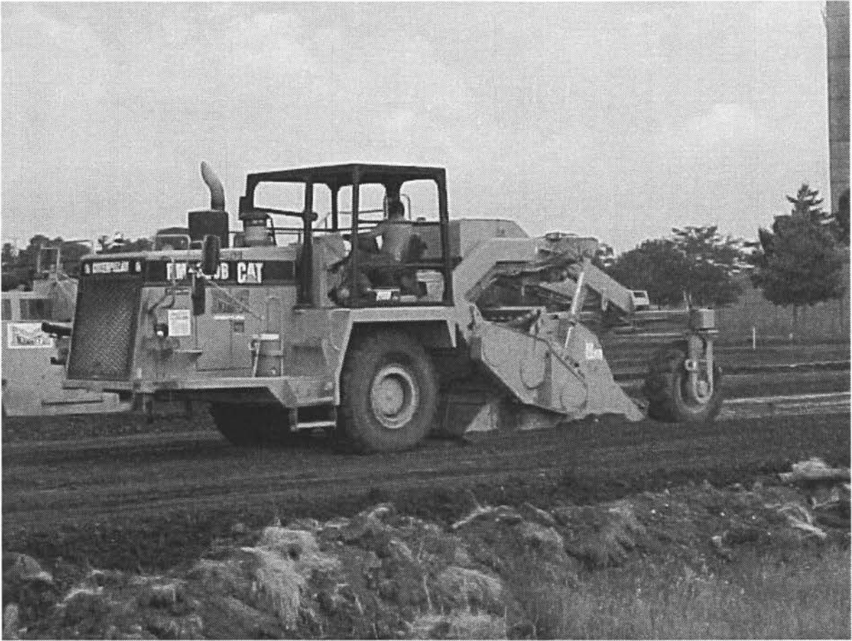
Figure 1. Typical Pulvamixer Used for On-Site Mixing
