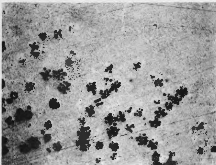
Figure 5. Lower Part of the Silver Phase in a Uranium - Silver Melt. (Magnification - 200X)
