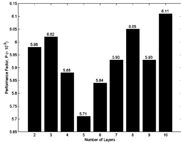
**Fig. 5** Performance parameter for case [01]. The parameter  $P$  measures the agreement between actual and estimated internal temperatures. Results show that a five-layer network has better performance.
