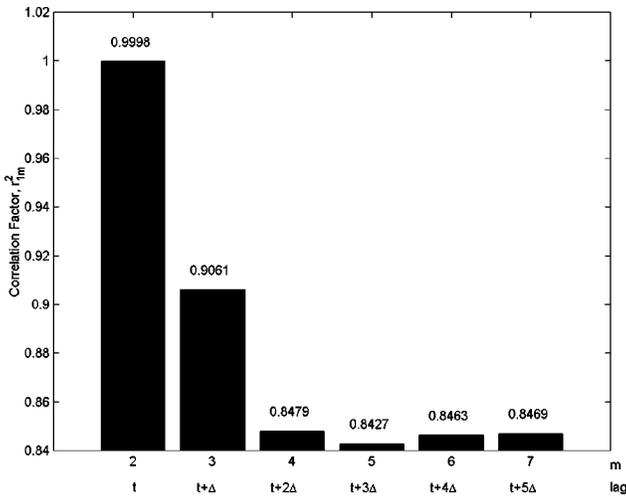
**Fig. 4** Results of covariance matrix criterion. The vertical axis corresponds to the square of the correlation coefficients of the covariance matrix  $r_m^2$ . The horizontal axis corresponds to the lag in terms of  $\Delta$ .
