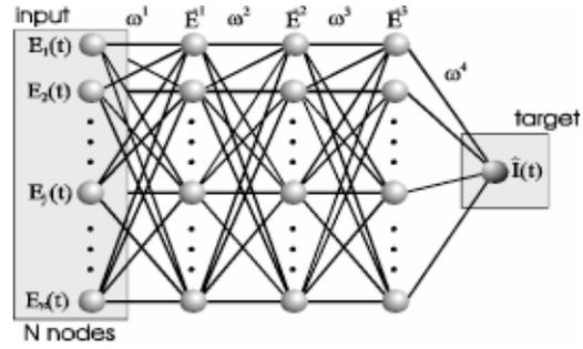
Fig. 3 Five layer feedforward network architecture. The output  $\hat{I}(t)$  is the estimated internal temperature at time  $t$ . The input  $\mathbf{E}(t)$  is composed of simultaneous and lagged observations of external temperature. The matrix  $\omega^i$  contains the weight factors between the layer  $\mathbf{E}^i$  and the previous layer.
