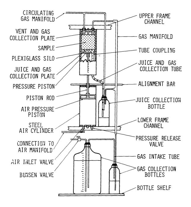
Figure 1.4. Component parts of each laboratory silo. The top vent plate contains parts for the circulating gas and gas manifold. The gas collection plate is placed above the sample. The juice collection plate rests on the pressure piston and contacts the bottom of the sample. The 1 mm rubber gasket between the upper part of the silo and the 6 mm 0-ring surrounding the pressure plate provide an airtight seal
