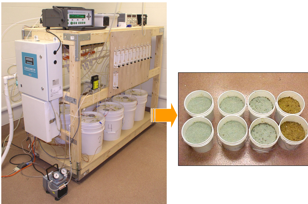
Figure 2. Photographs of the laboratory setup for evaluating efficacy of air emission mitigation strategies. Pictured to the right is topical application of zeolite on laying hen manure at various dosages.
