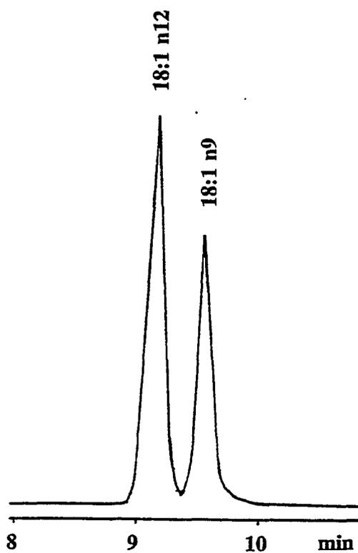
Figure 3. Separation of phenylethyl petroselinate and oleate on a DB-23 15-M capillary column (J&W, Deerfield, IL) operated isothermally at 220°C with helium as carrier gas at 1 mL/min
