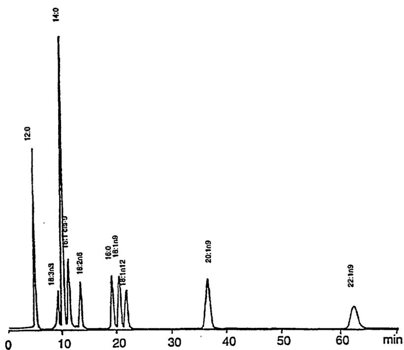
Figure 1. Separation of phenylethyl esters by high-performance liquid chromatography on a C-18 column with methanol/water 95:5 (vol/vol) at 2 mL/min.
