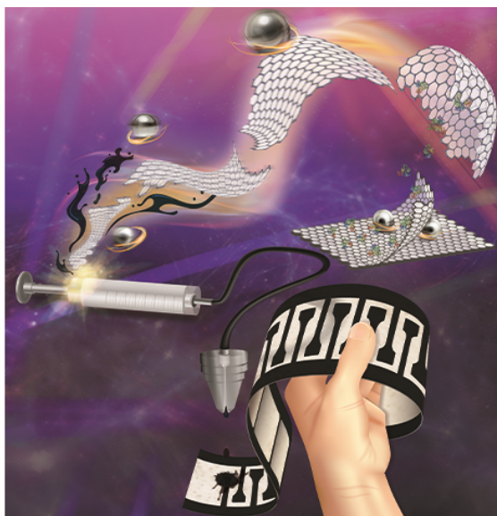
Figure 0.1 Schematic representation of graphene production through wet ball milling for fabrication of inkjet-printed patterns.
