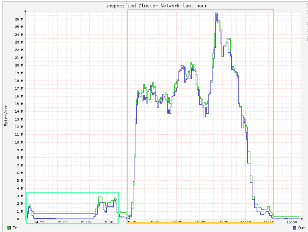
Fig. 26. Network utilization. Note the minimal use by the MapFile store (left) compared to the HBase store (right).
