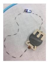
Figure 1 Electronic components in a series circuit
