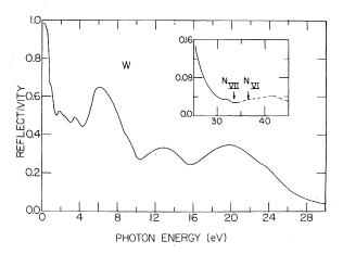
FIG. 1. Reflectivity spectrum of W. The high-energy region is shown in the insert.
