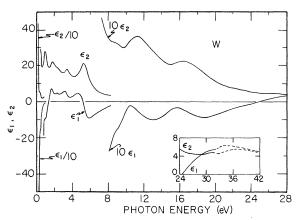
FIG. 3. Real and imaginary parts of the dielectric function of W. The high-energy region is shown in the insert.
