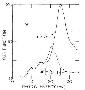
FIG. 5. Electron-energy-loss functions:  $\text{Im}(-1/\tilde{\epsilon})$  is the volume-loss function and  $\text{Im}[-1/(\tilde{\epsilon}+1)]$  is the surface-loss function.
