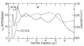
FIG. 2. Absorptivity (A=1-R) of W below 7 eV (right-hand scale). The interband  $\epsilon_2$  is also shown (left-hand scale).
