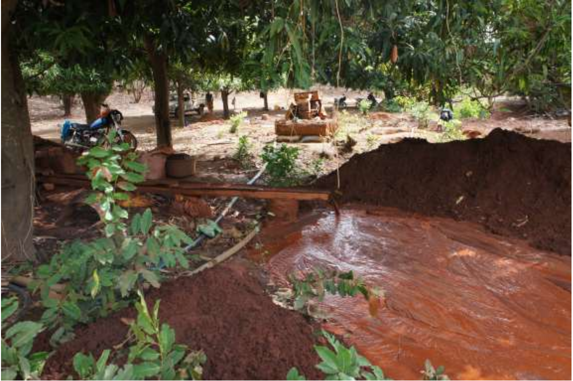
Figure 2.8 Small-scale mining near the Djendji village showing a sluice box and the mine tailing. Image taken in 2015 by K. Boyer Ontl.
