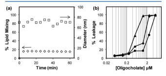
**Figure 3.** (a) Percent lipid-mixing and the size of the POPC/POPG LUVs upon the addition of **5**. [**5**] = 2.5  $\mu$ M, [phospholipids] = 54.0  $\mu$ M. (b) Percent leakage of glucose at 30 min induced by **1** ( $\blacktriangle$ ), **5** ( $\blacklozenge$ ), and **12** ( $\blacklozenge$ ) from POPC/POPG LUVs. [Phospholipids] = 104  $\mu$ M.
