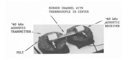
EMPTY RUBBER CHANNEL CONNECTED BETWEEN ACOUSTIC TRANSMITTER AND RECEIVER.
