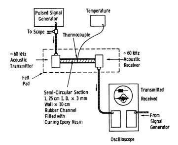
Figure 1. Schematic of experimental apparatus for determining the acoustical properties of curing resin filled with hollow spheres.
