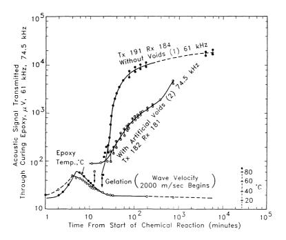
Figure 4. Changes in the acoustic signals transmitted through curing epoxy with and without artificial voids.
