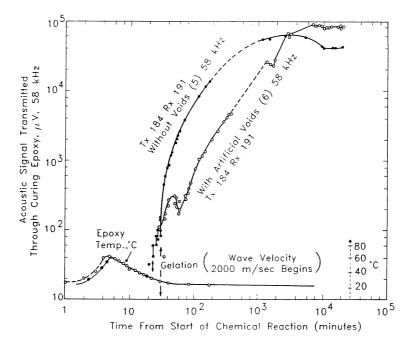
Figure 6. Changes in the acoustic signals transmitted through curing epoxy with and without artificial voids.
