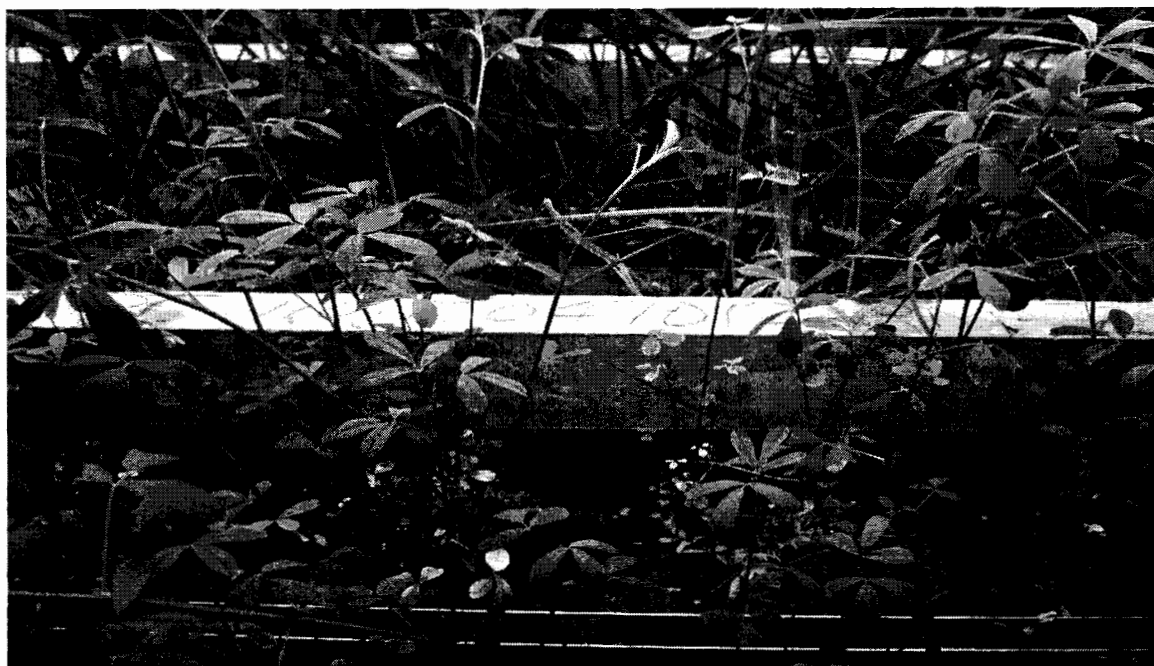
Figure 1: Side (picture above) and top (picture below) view of the channels: Channels 1 and 2 are alfalfa and channel 3 is grass. Lighting is provided by a pair of tube lights for each channel. PCE solution enters from a glass tank on the left side and is collected in a bottle on the right side.
