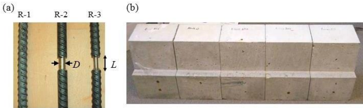
Figure 22. (a) Bare #4 reinforcing steel specimens and (b) concrete test specimens consisting of either #4 or epoxy-coated #6 reinforcing steel
