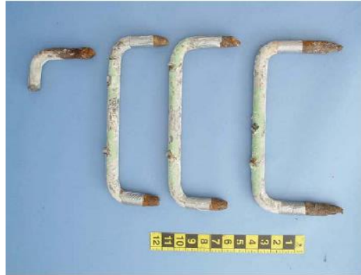
Figure 1. Corroded conditions of several U-bolt anchors that were extricated from concrete bridge barrier rail (NTSB 2010)
