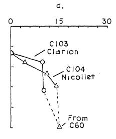
Figure 29. Bulk density profiles for soils on upper convex slopes of the JSS traverse in the Jewell bog watershed
