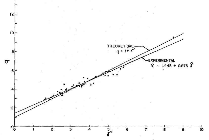
Figure 10. Variation in the geometry of the dimensionless graph resulting from selection of parameters  $\hat{q}$  and  $\hat{\gamma}$ , in accordance with the regression equation  $\hat{q}=1.445+0.873$   $\hat{\gamma}$
