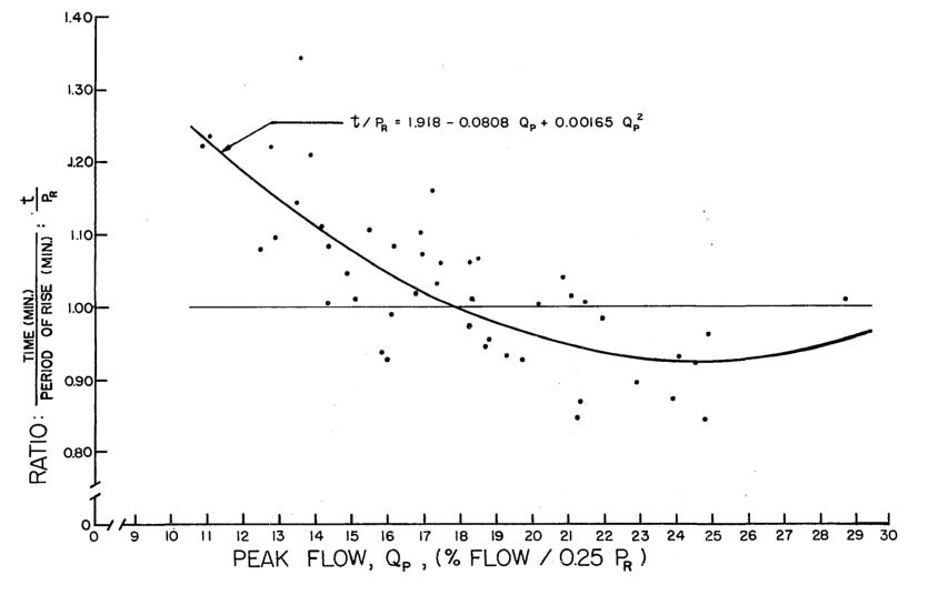
A comparison of the variances from regression for the regression line (Equation 22) and the linear model,  $t/P_R = 1$ , showed a significant reduction in the sum of squares by using the curvilinear line. The statistical evidence supports the observations previously discussed; namely, that for the fitted curves, the value of  $t/P_R$  at the peak is not a constant for each watershed but varies with the magnitude of the peak ordinate in a manner described by Equation 22.
