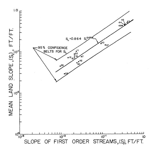
Equation 13 furnishes a simple relationship whereby an estimate of the mean land slope can be obtained from the slopes of the first-order streams. The empirical results are valid only within the range of data included. Obviously, it is unrealistic for  $S_L$  to exceed  $S_1$  as Equation 13 provides. However, because of the ease of measurement of  $S_1$ , additional work is warranted to establish the relation more concretely.
