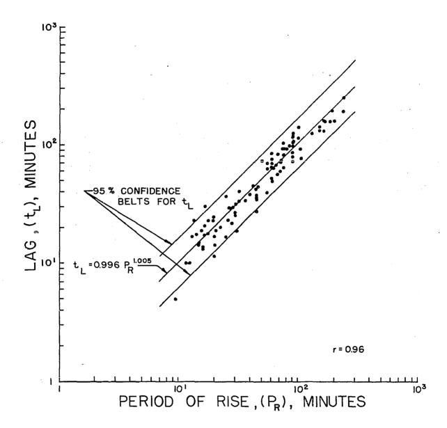
defines the functional relationship between the two variables (15, p. 106). The variances from regression for the  $t_L$ -values and  $P_R$ -values were approximately equal. The percent standard errors of estimate or coefficients of variation were calculated to be 27.1 percent and 25.7 percent, respectively.
