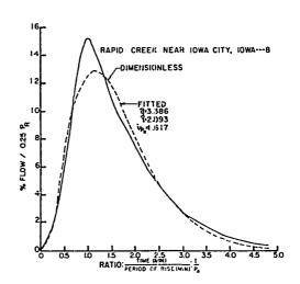
Figure 37. Dimensionless graphs and fitted two-parameter gamma distributions for watersheds 9, 10, 11, and 12
