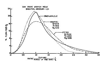
Figure 41. Dimensionless graphs and fitted two-parameter gamma distributions for watersheds 25, 26, 27, and 28
