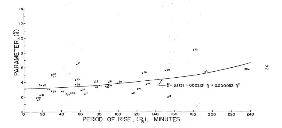
initial attempt to fit a linear regression model of the form,  $\hat{\gamma}=a+bP_R$ , proved unsuccessful. However, the use of a curvilinear regression model,  $\hat{\gamma}=a+bP_R+cP_R^2$ , resulted in a significant reduction in the sum of squares of deviations from regression over that obtained with the linear model. The quadratic equation obtained by the method of least squares is of the form
