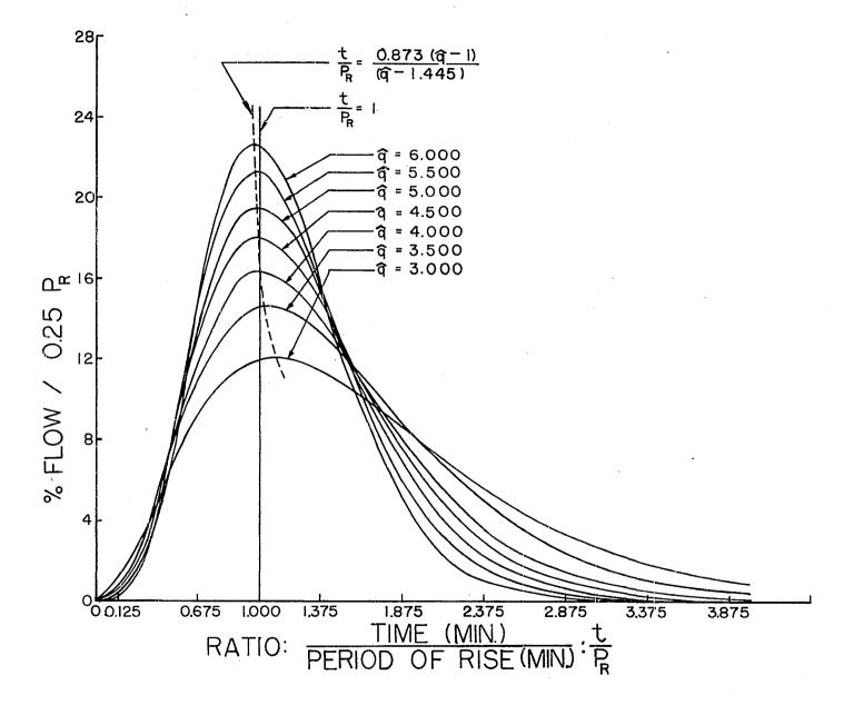
Figure 11. Inconsistencies in the positioning of the peaks of the dimensionless graphs described by the fitted gamma distributions
