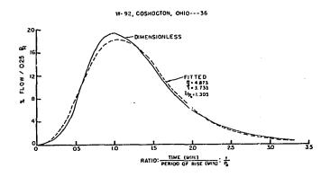
Figure 44. Dimensionless graphs and fitted two-parameter gamma distributions for watersheds 37, 38, 39, and 40
