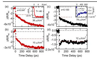
FIG. 3. Ultrafast THz pump probe scan at different pump fluences for (a),(b) x = 0.047 and (c),(d) x = 0.1 samples. All traces are taken in the superconducting state at T = 4.1 K. Inset of (a) the initial dynamics. Inset of (c) The THz dynamics in LuNi<sub>2</sub>B<sub>2</sub>C at pump fluence of 40  $\mu$ J/cm<sup>2</sup>.
