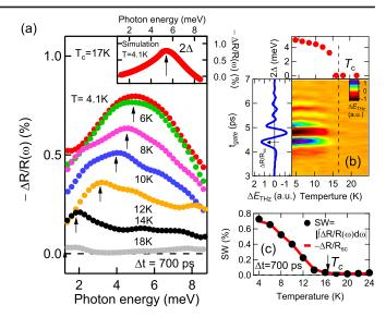
FIG. 2. (a) THz differential reflectivity spectra (dots) for the x = 0.047 sample at 700 ps. The cusp peak marked by black arrows reflects  $2\Delta_{SC}$ . Inset shows the MB simulation (see text). (b) Temperature-dependent  $\Delta E/E$  THz transients. Left panel:  $\Delta E/E$  transient at 4.1 K. Top panel: temperature dependence of  $2\Delta_{SC}$ . (c) Temperature dependence of the integrated spectral weight and peak transient amplitude.
