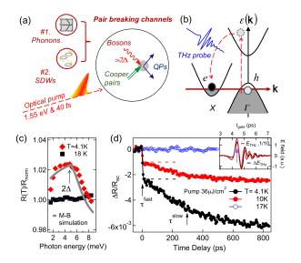
FIG. 1. Schematics of SC pair breaking channels, (a) and interband transitions, (b) after fs pump photoexcitation. (c) Static THz reflectivity spectra, normalized to the normal state spectra at 20 K, for underdoped x = 0.047 sample, at 4.1 and 18 K. Gray line shows the result of the Mattis-Bardeen theory. (d) Ultrafast THz dynamics for the above underdoped sample. Inset: The measured time-dependent THz field transients, with gate-time (blue arrow) t<sub>gate</sub> = 4.4 ps, at T = 4.1 K.
