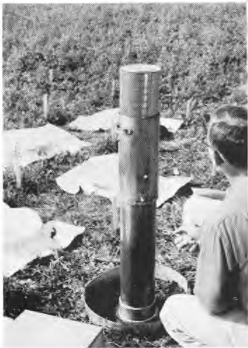
Fig. 1. Air permeameter in field use. In the background can be seen several areas previously moistened and covered with sheet aluminum.
