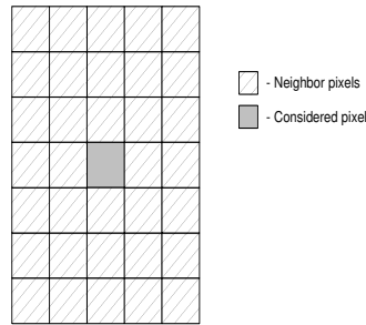
FIGURE 9. 7 \times 5 neighborhood used to remove false alarms from the GLR results in Figure 8.
