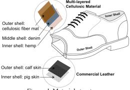
Figure 1. Material structures.
