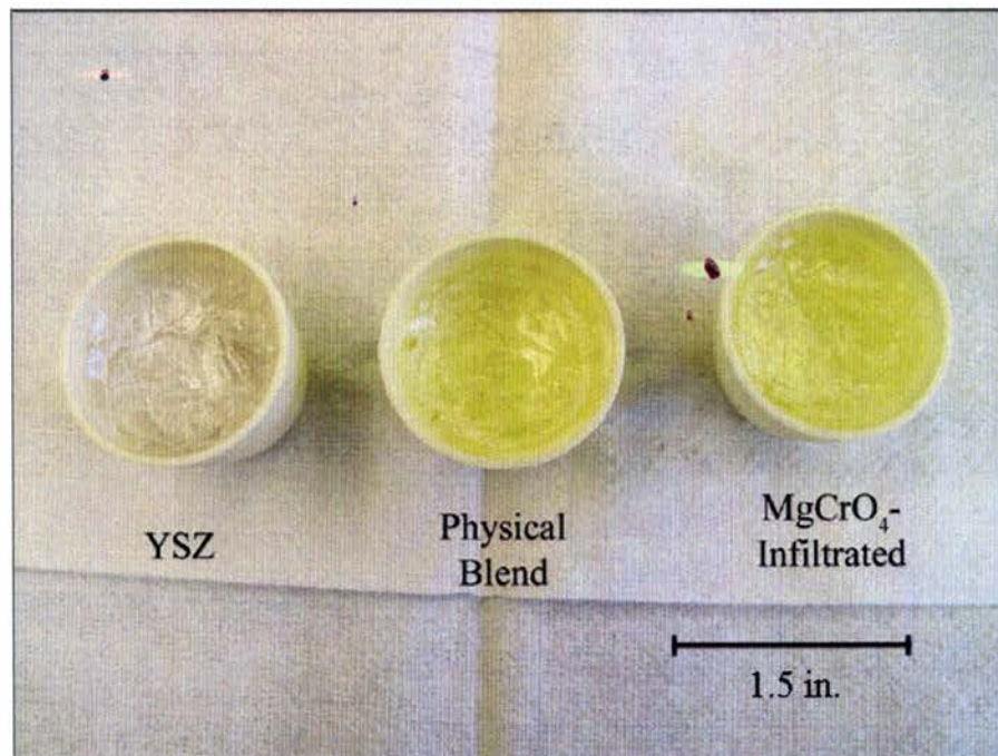
Figure 47. Crucibles of salt after 4-hour crucible test.
