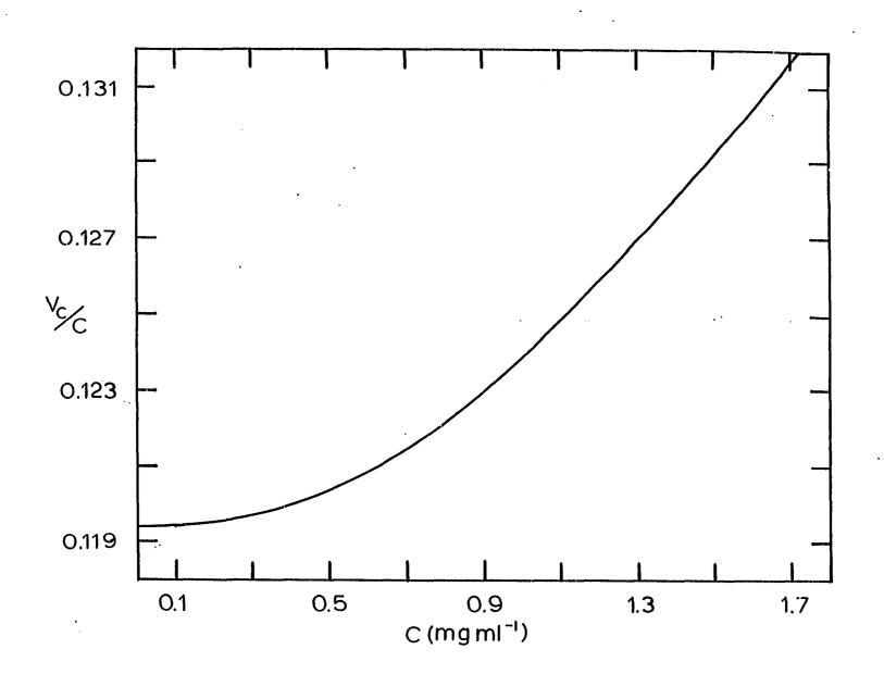
thirds of the curve. Therefore, in order to keep the relative variance at a reasonable level, samples of high concentration should be diluted such that the response of the sample is in the low region of variance of the calibration curve.
