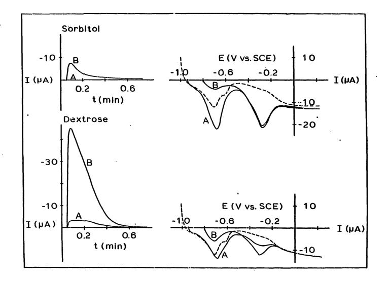
for both sorbitol and dextrose. These peaks can originate only from the adsorbed carbohydrates. When a period greater than 45 s was allowed to transpire before recording the I-E curves, the anodic peaks in the double-layer region were smaller than for 45 s, undoubtedly because of the slow desorption of the reaction products of the oxidation in the hydrogen region.
