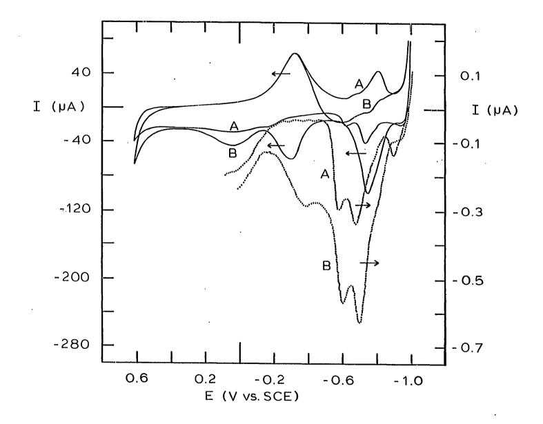
Figure V-8. Current-voltage curves for sorbitol at a platinum RDE by cyclic voltammetry and triple pulse voltammetry
