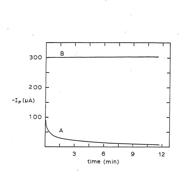
platinum electrode was repeatedly switched between 1.25 and 0.00 V to insure a clean electrode surface prior to recording the I-t curve at the constant potential 0.26 V. The signal for the TPA detection was observed to remain constant for 0.5 hr at which time the experiment was discontinued.
