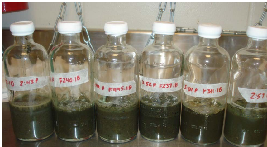
Figure 2. A set of samples after three days of incubation for the methane production rate assay.
