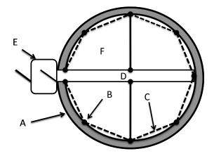
**Diagram 1. A circular, insulated tent layout for farrowing 4 sows** (diameter = 7.3m, height of perimeter wall = 1.8 m)
