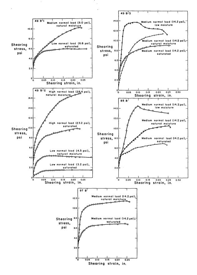
to an ultimate value before failure, and if the ultimate value rather than the maximum value is entered on the plot there is no sharp increase in strength. This decrease in shearing strength with increasing strain also occurs under certain conditions in other soils.
