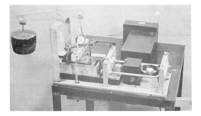
consolidation became so slow that further consolidation would be negligible (less than about 0.0003 inches per hour), a final reading was recorded on the data sheet. The time required was two hours or less for light loads and from four to six hours for the heavy loads.
