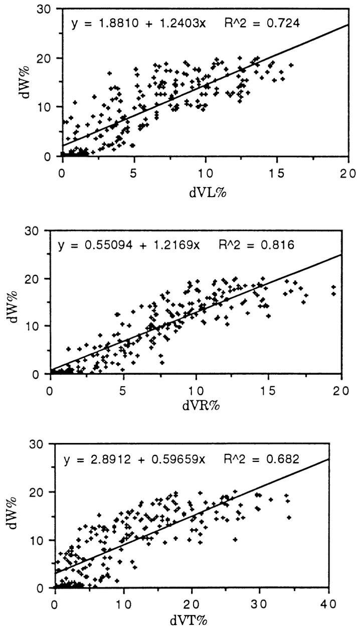
Figure 4-9. Relationship between percent weight loss (dW%) and ultrasonic velocity for specimens having percent weight losses 0%-20%. dVL%=percent reduction in longitudinal velocity; dVR%=percent reduction in radial velocity; dVT%=percent reduction in tangential velocity.
