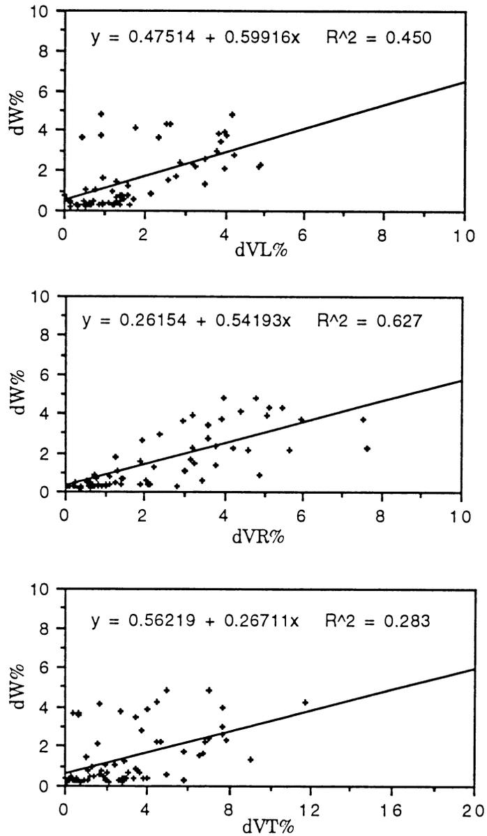
Figure 4-6. Relationship between percent weight loss (dW%) and ultrasonic velocity for specimens having percent weight losses 0%-5%. dVL%=percent reduction in longitudinal velocity; dVR%=percent reduction in radial velocity; dVT%=percent reduction in tangential velocity.
