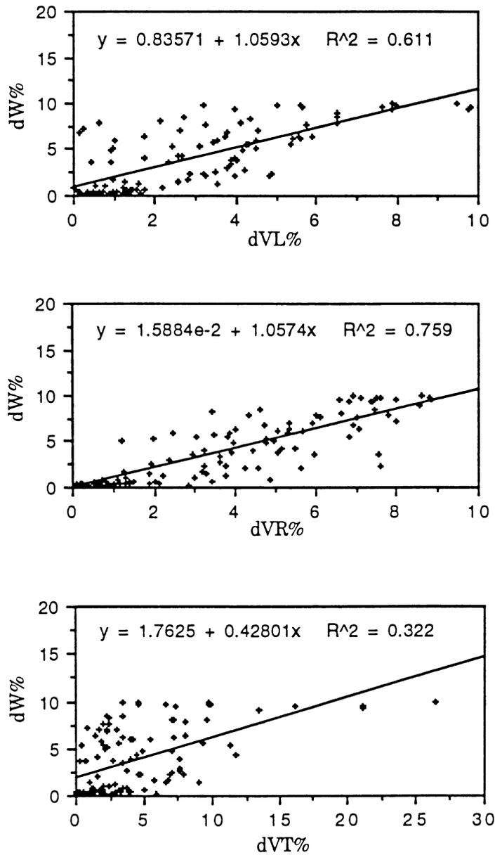
Figure 4-7. Relationship between percent weight loss (dW%) and ultrasonic velocity for specimens having percent weight losses 0%-10%. dVL%=percent reduction in longitudinal velocity; dVR%=percent reduction in radial velocity; dVT%=percent reduction in tangential velocity.
