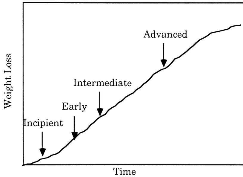
Figure 2-1. The continuum of the decay process under ideal decay conditions and its subdivision into several decay stages (Zabel 1992).
