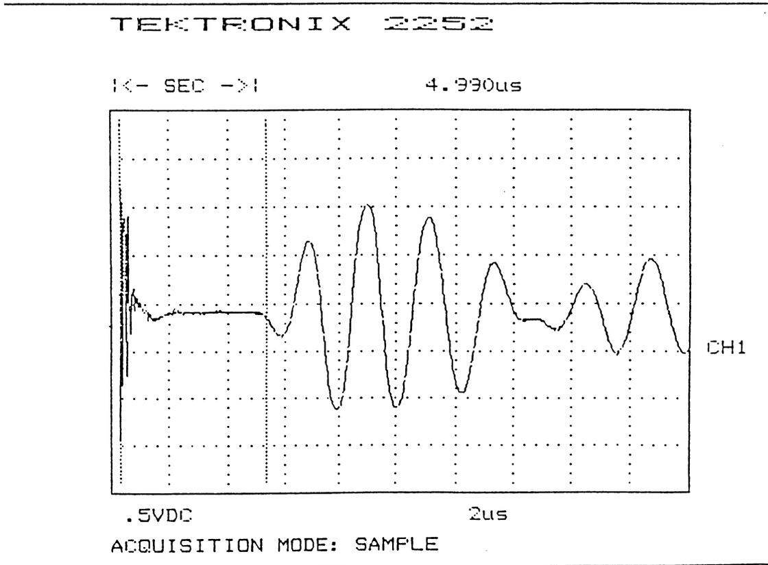
Figure 4-2. Determination of ultrasonic transit time
