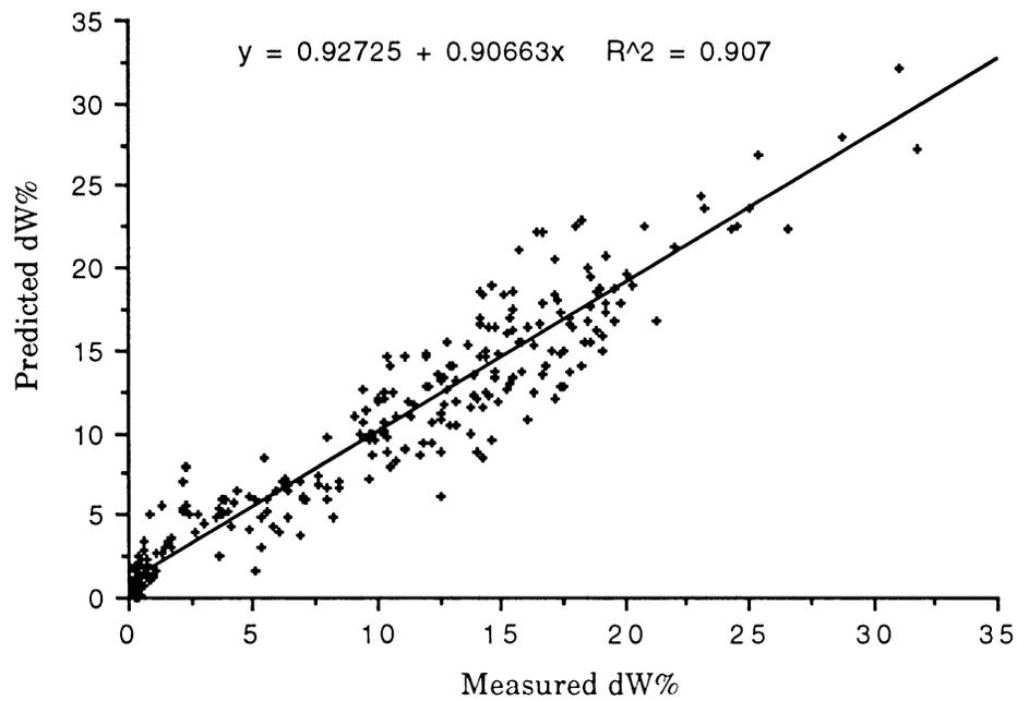
Figure 4-5. Relationship between predicted percent weight loss and measured percent weight loss for specimens weight loss ranging from 0%-32%.
