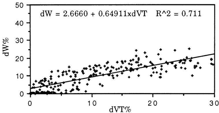
Figure 4-4. Relationship between percent weight loss (dW%) and ultrasonic velocity for specimens having percent weight losses 0%-32%. dVL%=percent reduction in longitudinal velocity; dVR%=percent reduction in radial velocity; dVT%=percent reduction in tangential velocity.
