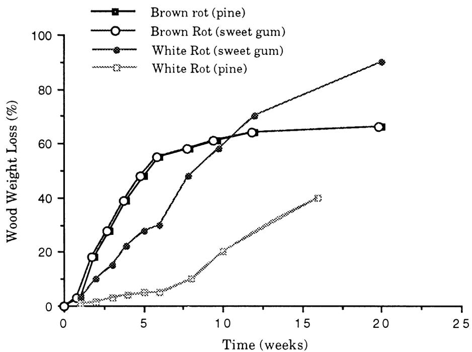
Figure 2-2. Relationships between time and weight loss as affected by type of decay and substrate (Zabel 1992)
