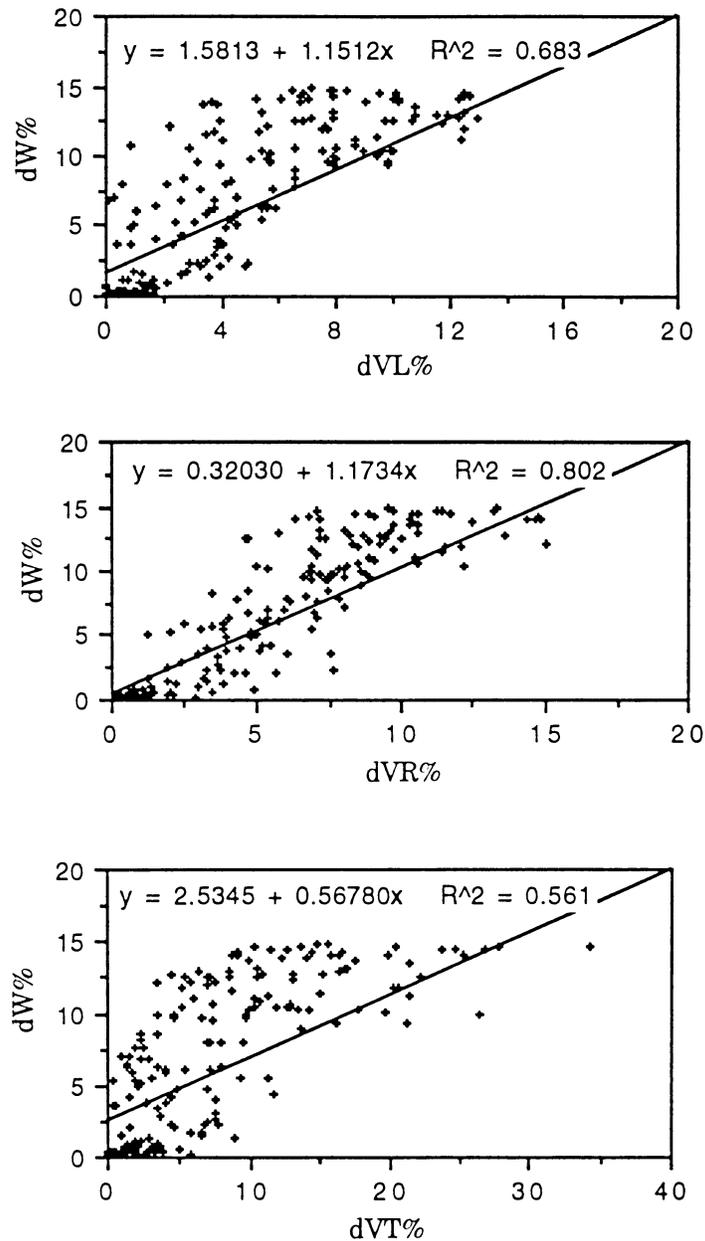
Figure 4-8. Relationship between percent weight losses (dW%) and ultrasonic velocity for specimens having percent weight losses 0%-15%. dVL%=percent reduction in longitudinal velocity; dVR%=percent reduction in radial velocity; dVT%=percent reduction in tangential velocity.
