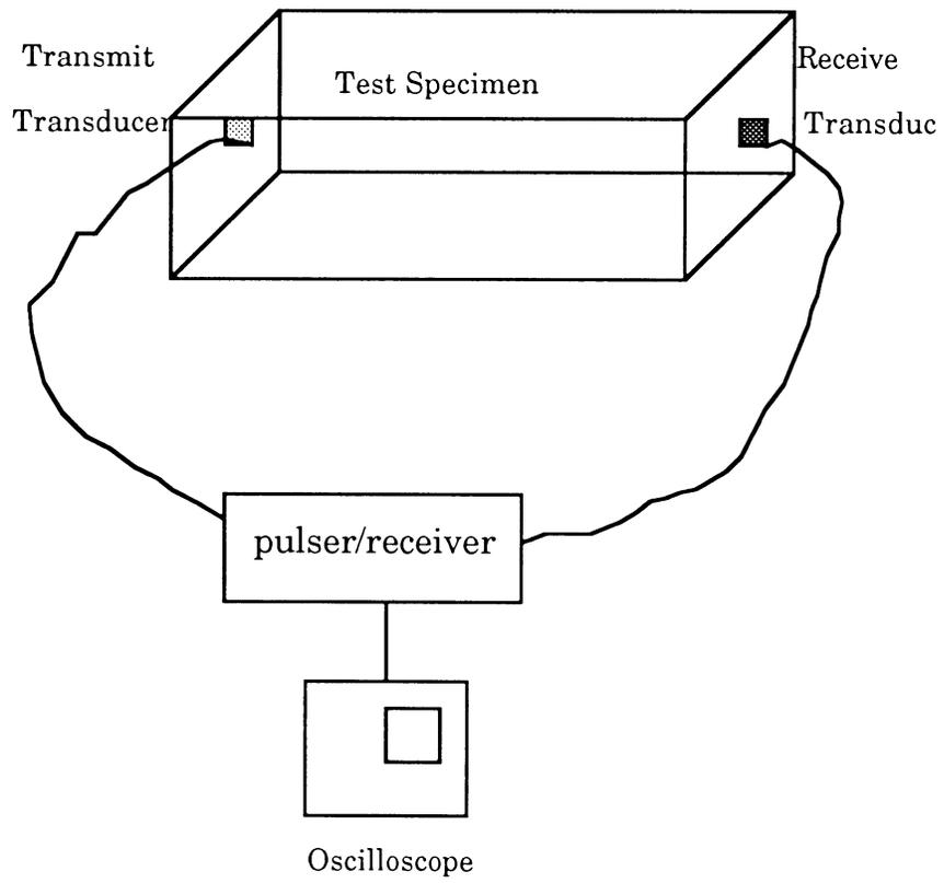
Figure 2-4. Ultrasonic wave velocity measurement.
