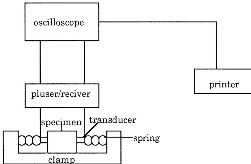
Figure 3-1. Schematics of ultrasonic pulse velocity measurement
