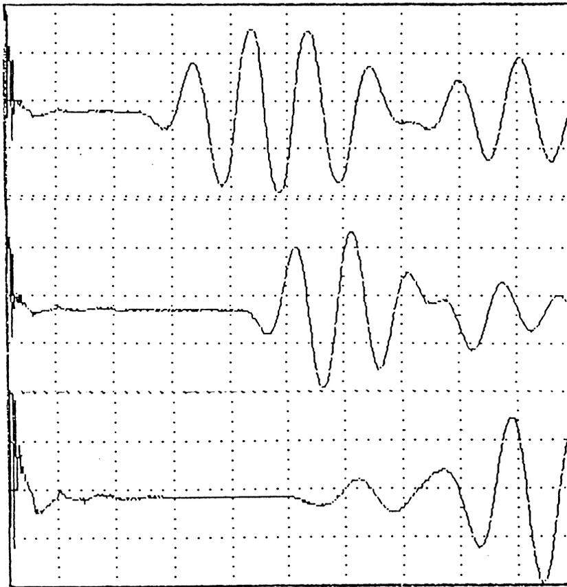
Figure 4-1. Ultrasonic waveforms in the longitudinal (top), radial (middle), and tangential (bottom) directions of ponderosa specimens
