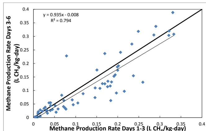
**Figure 2. Comparison of methane production rates of manure samples from 62 swine finishing operations on days 3-6 and days 1-3. The thicker black line represents a one-to-one line, the thinner black line the best fit line. The best fit line was not statistically different than the one-to-one line.**
