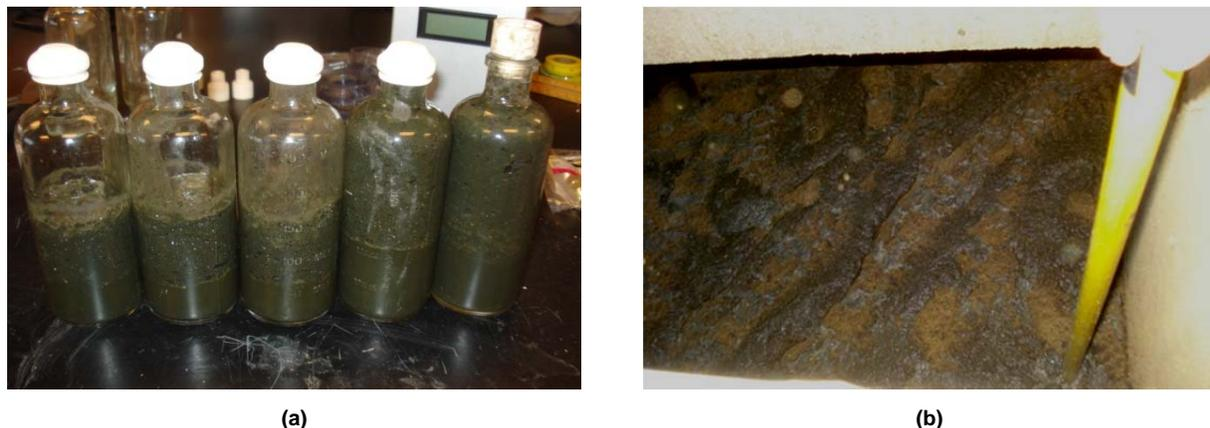
**Figure 1. Manure foam accumulation on the surface of swine manure samples during (a) an anaerobic incubation of swine manure in the lab and (b) in the pumpout of a deep-pit manure storage at a swine finishing facility.**
