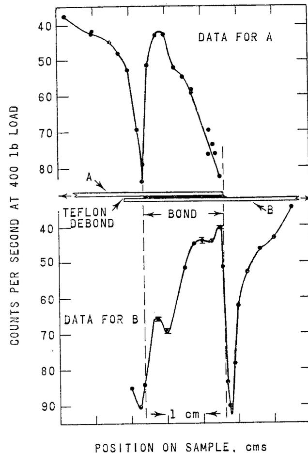
Fig. 4. Diffracted intensities for surfaces A and B of adhesively bonded 1/32" thick aluminum strips. Longitudinal tensile stress increases with decreasing count rate. Constant angle method with 400 lb load.
