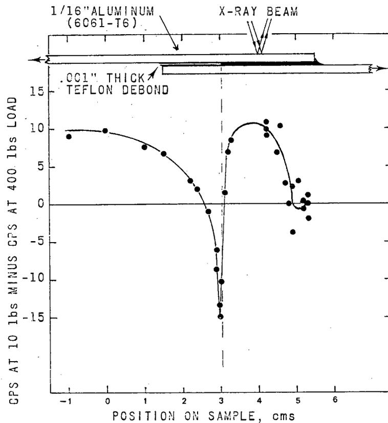
Fig. 2. Counts per second (CPS) vs. position for adhesive joint between aluminum strips 1/16" thick, with teflon debond. Constant angle method, with change in load of 390 lbs (7.6 ksi, 52.4 MPa). Increasing CPS at 10 lbs minus CPS at 400 lbs corresponds to increasing longitudinal tensile stress
