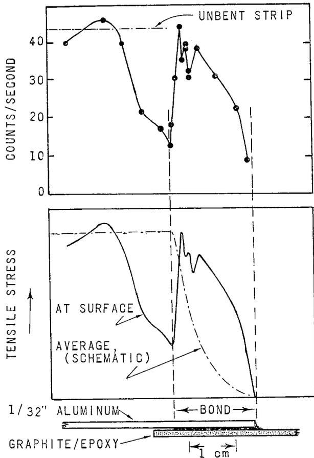
Fig. 6. Adhesive joint between 1/32" aluminum and 6-ply graphite/epoxy unidirectional composite. Upper plot: aluminum diffraction in counts per sec by constant angle method. Lower plot: surface stresses from the diffraction data compared with average stress throughout adherend cross section in the absence of bending (dot-dash line, schematic)
