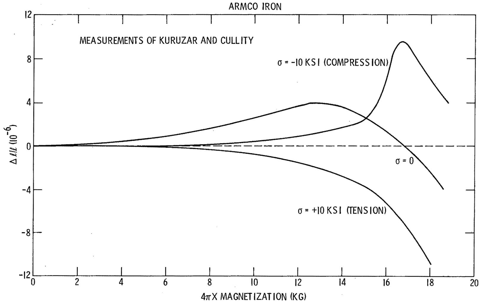
Fig. 7. Stress dependence of magnetostriction of polycrystalline iron.
