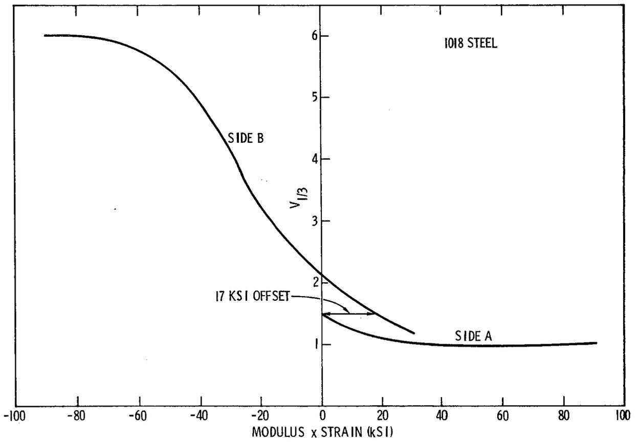
Fig. 10. Variation of  $V_{1/3}$  with stress.
