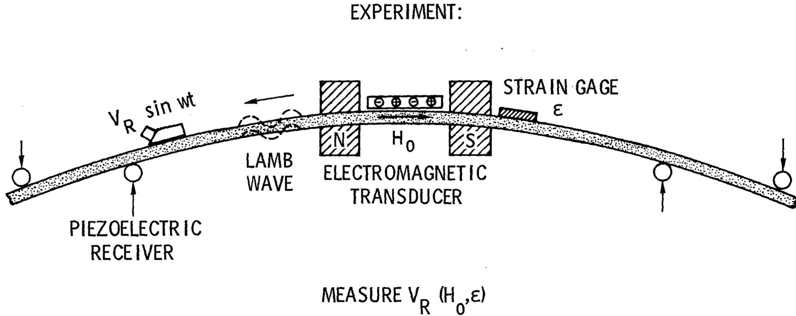
Fig. 8. Experimental apparatus for measuring stress dependence of transducer efficiency.
