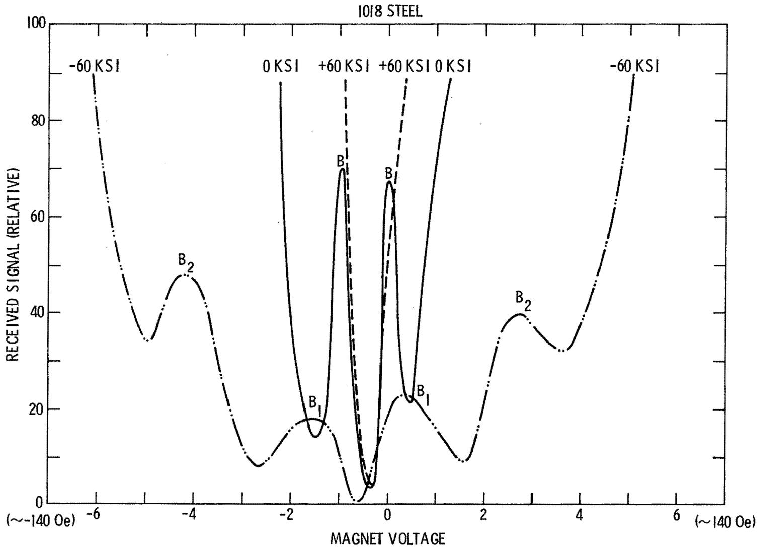
Fig. 9. Transducer efficiency versus magnetic field (volts) for tensile and compressive stresses.
