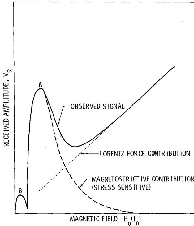
Fig. 2. Experimental configuration for measuring magnetic field dependence of electromagnetic transducer efficiency and schematic data.
