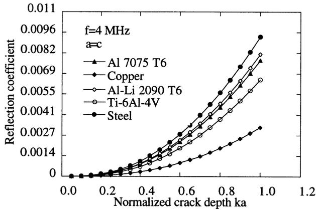
Fig 4. The reflection coefficient vs. the normalized crack depth on alternative materials.
