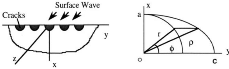
Fig 2. The schematic of a planar distribution of surface cracks and the geometric quantities of a semi-elliptic surface crack.
