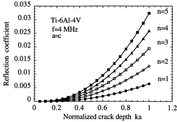
Fig 3. The reflection coefficient vs. the normalized crack depth for varying the number of cracks.
