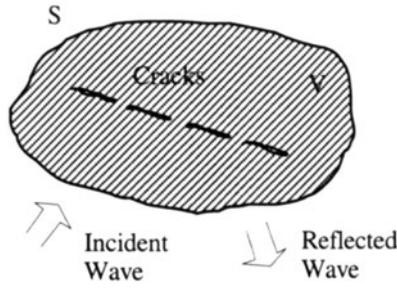
Fig 1. The schematic of a planar distribution of cracks.
