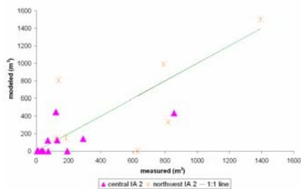
Figure 3. Measured versus modeled vegetated infiltration basin outputs.
