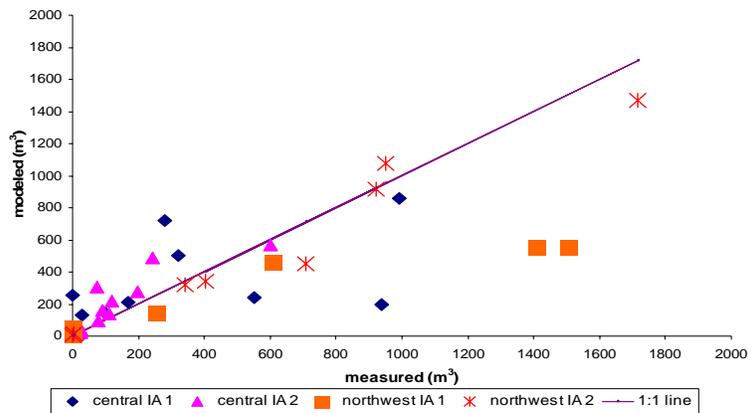
Figure 2. Measured versus modeled solid settling basin outputs.
