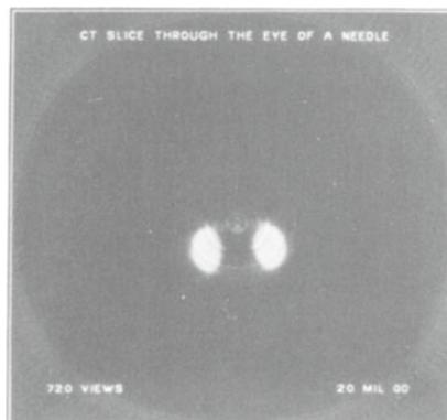
Figure 8. CT slice through the eye of a needle.
