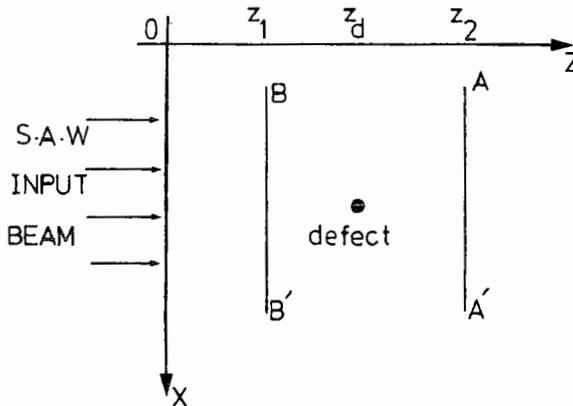
Fig. 8 Recording configuration for defect characterisation.
