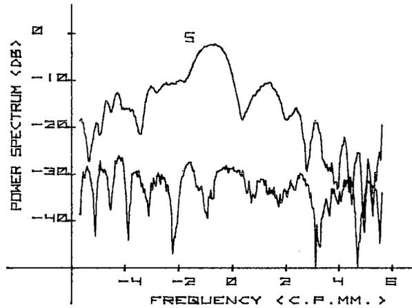
Fig. 13 Length determination of a rectangular slot defect.
