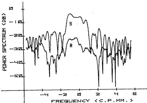
Fig. 12 Sizing of a circular shaped defect.
