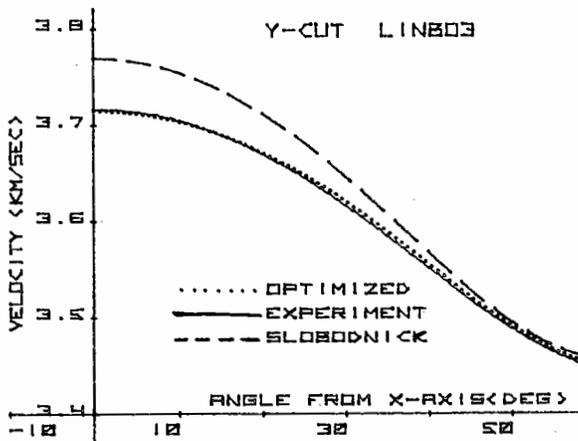
Fig. 7 Comparison between the experimental velocity curve and the computed curve obtained using the revised elastic constants for YX Lithium Niobate.
