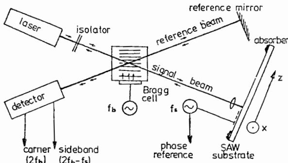
Fig. 1 Schematic of phase sensitive laser probe.
