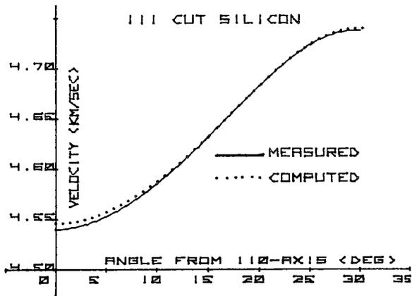
Fig. 4 Measured and theoretical velocity characteristics for (111) silicon
