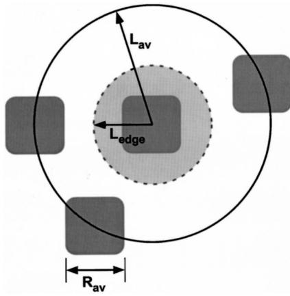
FIG. 3. Schematic showing the key linear dimensions for a typical island distribution: The mean separation between island centers,  $L_{av} = (N_{av})^{-1/2}$ ; the mean island edge length,  $R_{av} = \theta^{1/2}L_{av}$ ; and the mean separation between island edges,  $L_{edge} = L_{av} - cR_{av} = (1 - c\theta^{1/2})L_{av}$ , where  $c$  is of order unity.
