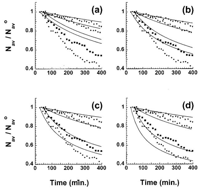
FIG. 4. Best fits to the family of data for the experimental coarsening kinetics with  $F = 0.003$  ML/s [Fig. 2(c)] from the rate equations with various  $\alpha = 1.0$  (a); 1.25 (b); 1.5 (c); 1.75 (d). Solid symbols show experimental data, and solid curves show predictions from Eq. (8).
