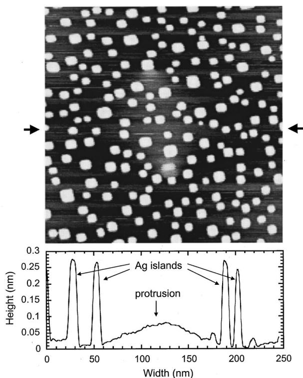
FIG. 7. Top: STM image of a 250 nm $\times$ 250 nm region showing 0.18 ML of Ag deposited on Ag(100). Bottom: Cross-sectional height profile taken horizontally through the center of the image (at a level indicated by the arrows), and spanning the oblong-shaped central protrusion.
