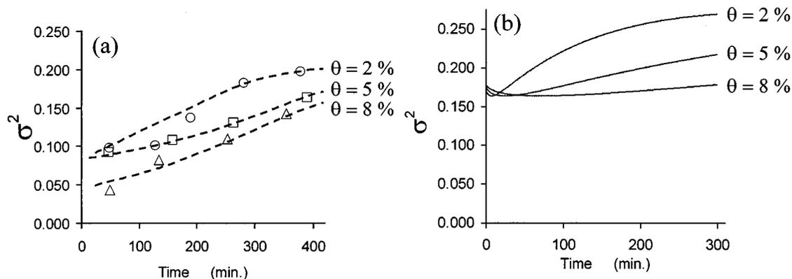
FIG. 6. Evolution of the variance,  $\sigma^2$ , for three cases corresponding to experiments with  $F=0.003$  ML/s and coverages of 0.02, 0.05, and 0.08 ML. (a) Estimates from experimental data (symbols), where dashed lines are shown as a guide to the general trend. (b) Rate equation predictions using an initial shape for the island size distribution,  $f_0(x)$ , with a variance of 0.18, as described in the text, and using  $\theta$ - and  $s_{av}^0$ -values consistent with experiment.
