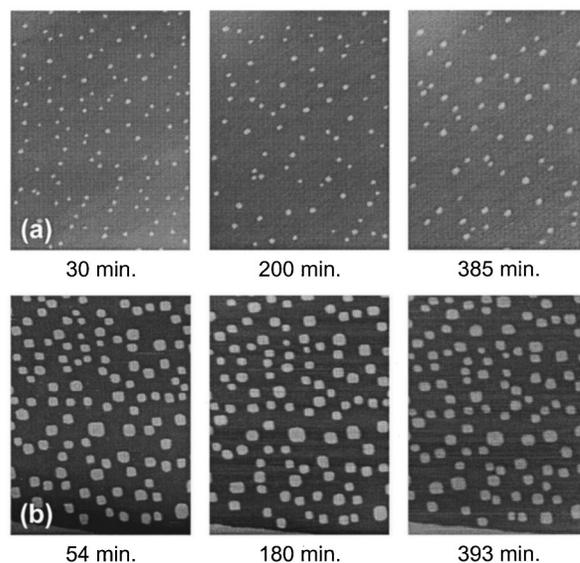
FIG. 1. Sequences of STM images of the ripening of Ag island distributions on Ag(100) for two coverages: (a)  $\theta=0.02$  ML, with  $s_{av}^0=60$  atoms; (b)  $\beta=0.21$  ML with  $s_{av}^0=510$  atoms. All images are  $150 \text{ nm} \times 100 \text{ nm}$ .
