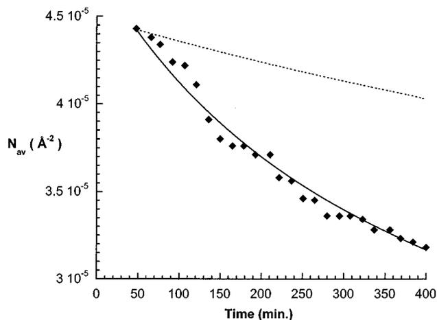
FIG. 8. Experimental data (solid symbols) for the coarsening kinetics for the region displayed in Fig. 7. Rate equations with the modified choice of parameters  $D_0=250 \text{ \AA}^2/\text{s}$  and  $\alpha=1.5$  (solid curve) fit observed behavior, in contrast to those with the previous choice  $D_0=50 \text{ \AA}^2/\text{s}$  and  $\alpha=1.5$  (dashed curve).
