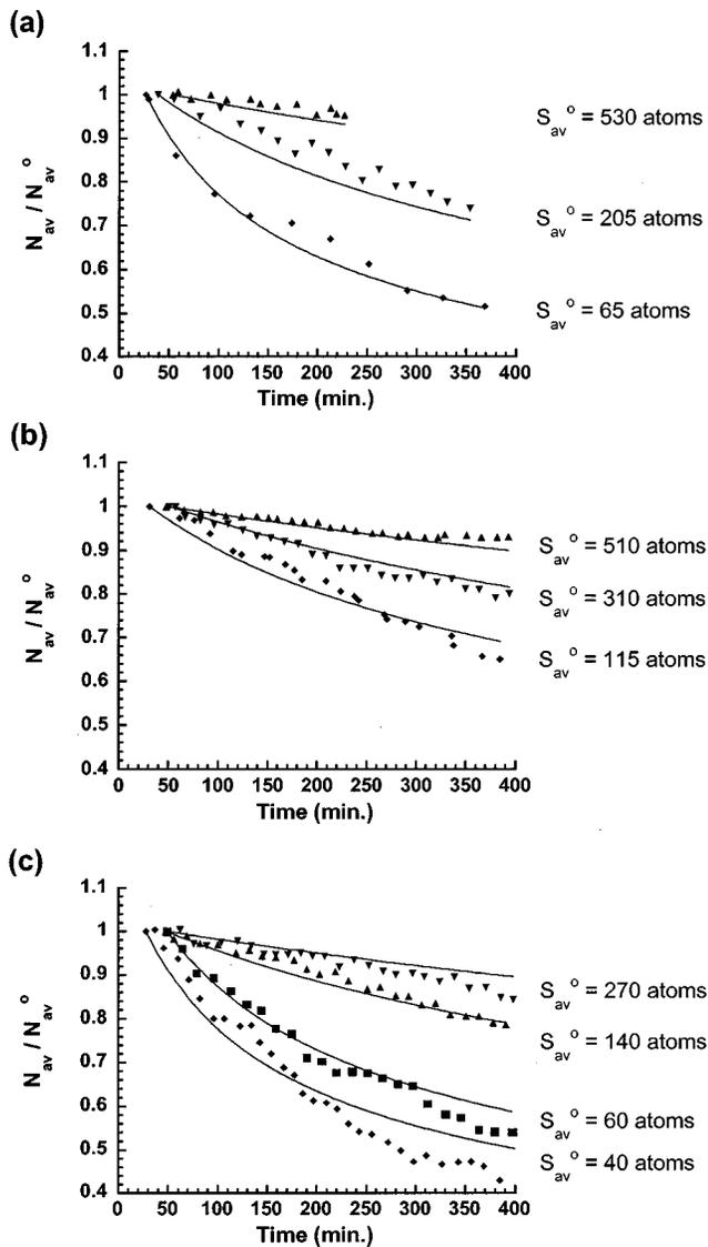
FIG. 2. Families of data illustrating the coarsening kinetics for three different fluxes: (a)  $F=0.011$  ML/s; (b)  $F=0.006$  ML/s; (c)  $F=0.003$  ML/s. Data points for each STM experiment are shown as various solid symbols labeled by  $s_{av}^0$ -values. Corresponding behavior predicted from Eq. (8) with  $\alpha=1.5$  and  $D_0=50 \text{ \AA}^2/\text{s}$  is shown as solid curves.
