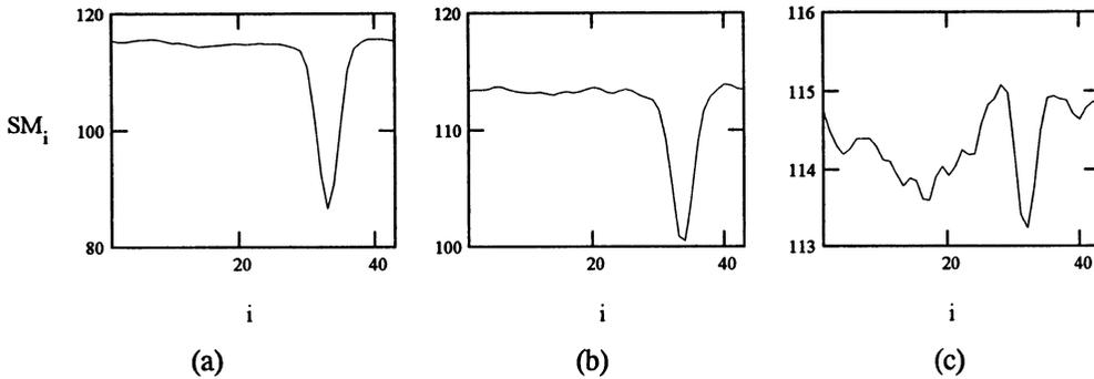
Figure 5 Sum of the magnitude under the magnitude curve for (a) 28 (b) 18 and (c) 8 mils long fatigue cracks.
