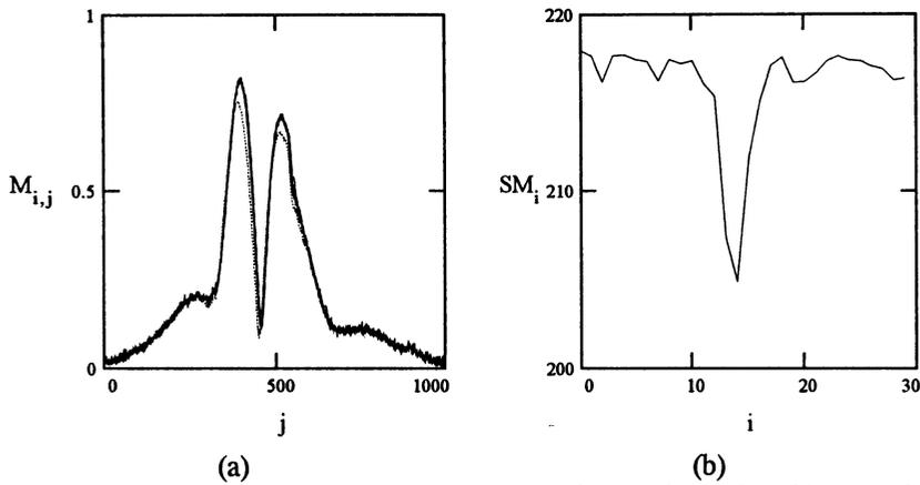
Figure 4 (a) Overlap of magnitude curves around a notched edge (b) sum of the magnitude under the magnitude curve.
