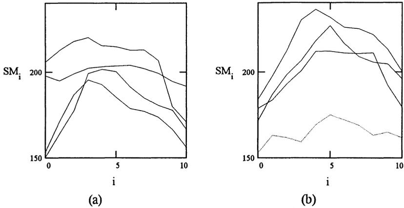
Figure 6 Sum of the magnitude under the magnitude curve for (a) inner edges and (b) outer edges of the e-hole. The dotted line indicates a 20 mils long EDM notch at the corner of the e-hole.
