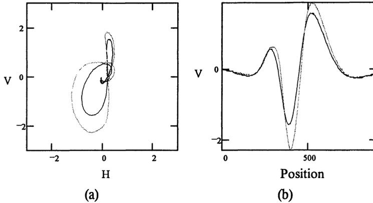
Figure 3. Eddy current signals on (a) the impedance plane and (b) vertical channel from a notch-free edge (dotted line) and a notched edge (solid line).
