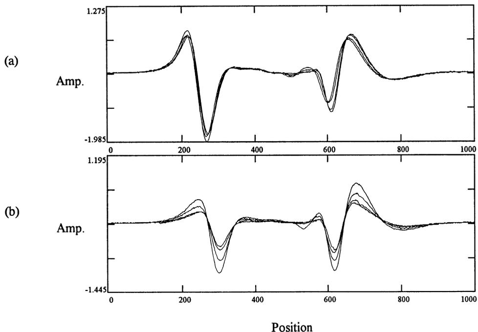
Figure 2. (a) Notch-free edge signals around a corner of the e-hole on the left side while notched edge signals on the right side (b) variation of notch-free edge signals as probe moves away from the corner of the e-hole.
