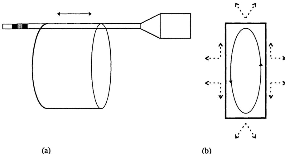
Figure 1. (a) Geometry of an e-hole and a probe tip in a corner of the e-hole; the arrow indicates the scan direction (b) the end-view from the probe tip: probe tip index pattern (bold line), compliance direction (dash line), and scanner index pattern (solid line).
