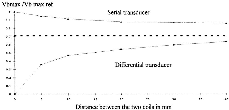
Figure 8 Influence of the distance between the two parts of a differential or « series » coil on the Barkhausen signal.
