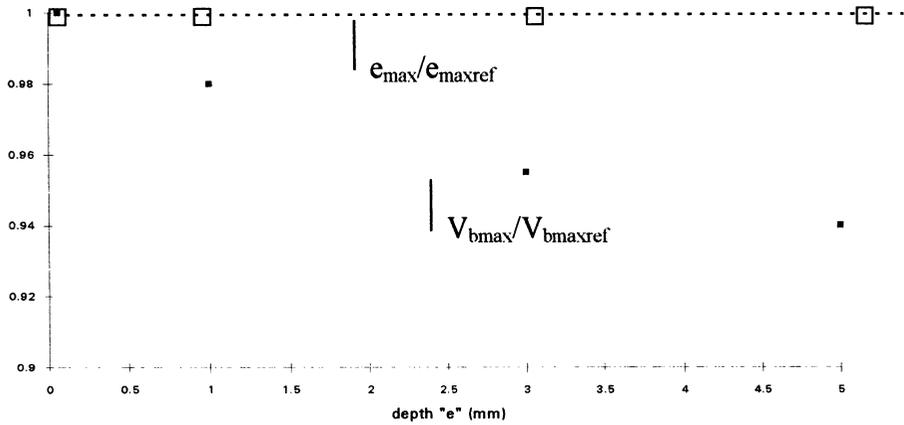
Figure 4 Influence of the distance between the coil and the sample.
