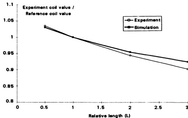
Figure 9 Comparison between experiment and simulation of RMS voltage variations related to the gap between turns.
