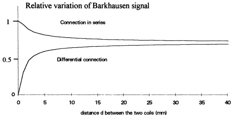
Figure 10 Numerical simulation of the voltage from two coils connected in series or in opposition in terms of distance between the two coils.
