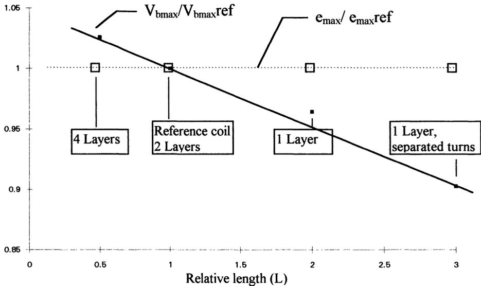
Figure 6 Influence of the relative length of the detection coil on the amplitude of the Barkhausen signal.
