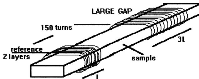
Figure 5 Constitution of the detection coil.
