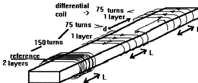
Figure 7 Two part coil: differential transducer.
