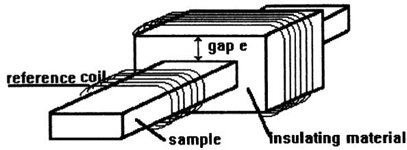
Figure 3 Coil at a distance « e » from the sample.
