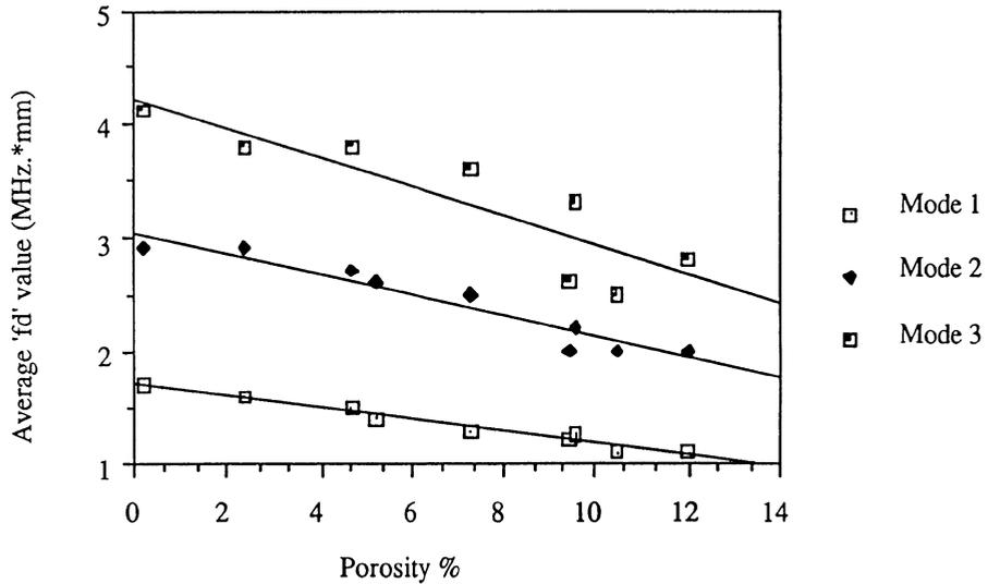
Fig. 2 The sensitivity of 'fd' shift feature to porosity.
