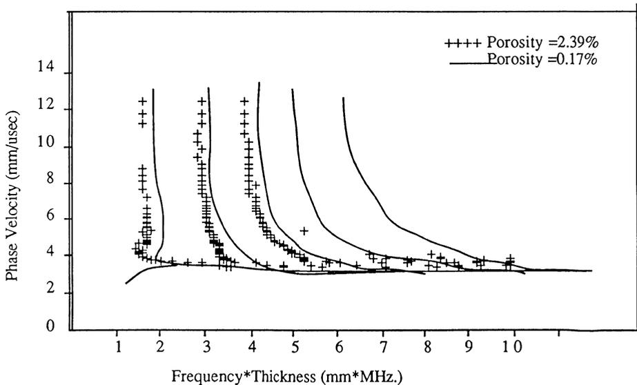
Fig. 3 The experimental dispersion curves for graphite-epoxy composites having two different levels of porosity.
