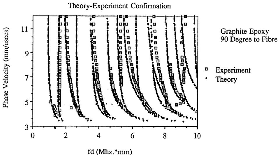
Fig. 1 The dispersion curves for a unidirectional graphite epoxy composite plate, with propagation across the fibers.
