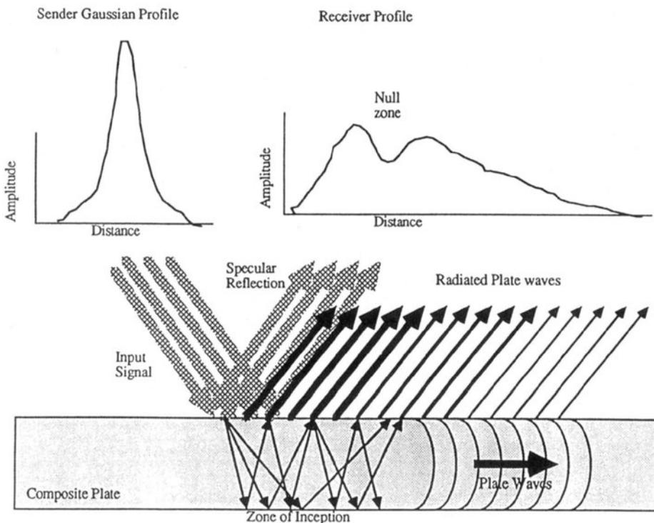
Fig. 5 The plate wave generation and reflection phenomena.
