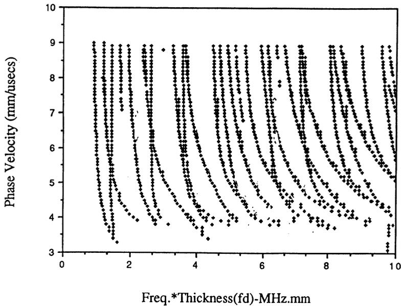
Fig. 4 Dispersion curves for a fiber mis-orientation of  $15^\circ$
