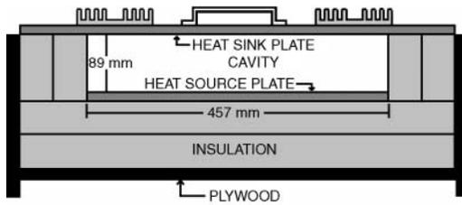
Fig. 1. Cross-section of laboratory heat flow chamber.
