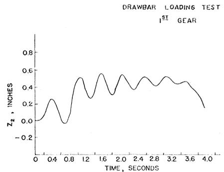
FIG. 24 Calculated curve of  $z_2$  vs. time.
