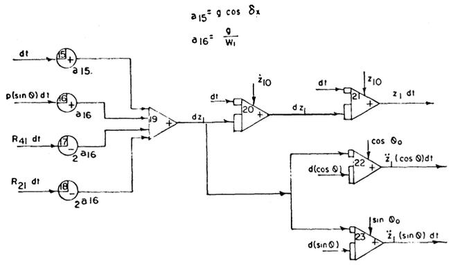
FIG. 10 Flow diagram for the generation of  $z_1$ .
