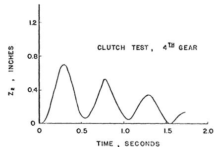
FIG. 20 Calculated curve of  $z_2$  vs. time.
