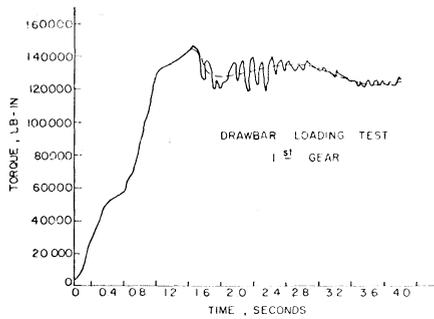
FIG. 21 Empirical curve of torque vs. time.
