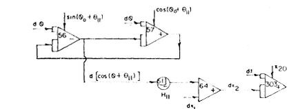
FIG. 16 Alternate flow diagrams for generation of rear wheel translational and rotational speeds and net thrust.
