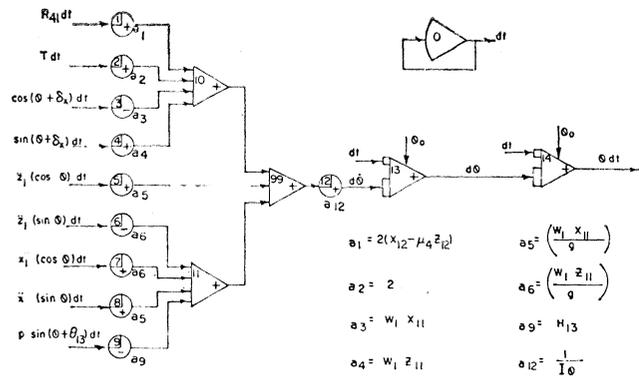
FIG. 9 Flow diagram for the generation of  $\theta$ .
