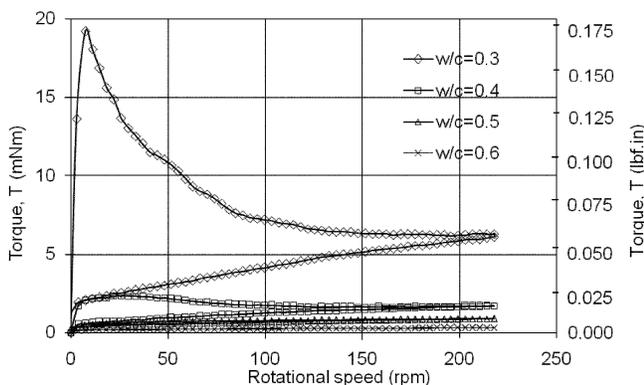
Fig. 4—Effect of  $w/c$  on paste rheological behavior.
