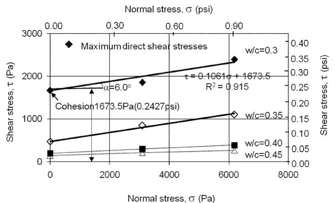
Fig. 3—Mohr-Coulomb failure curves of fresh cement pastes.
