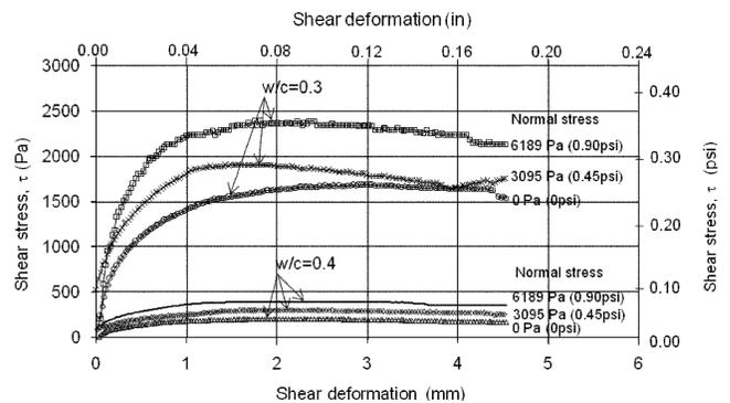
Fig. 2—Typical direct shear test results.
