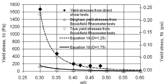
Fig. 6—Fitting of test data using Eq. (18).
