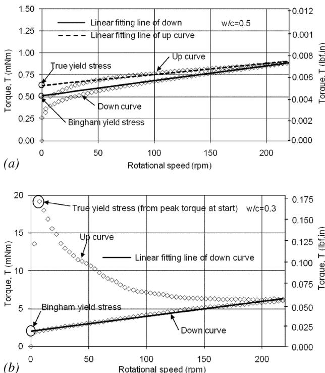
Fig. 5—True and Bingham yield stress defined from typical flow curves: (a) up-curve without peak value; and (b) up-curve with peak value.
