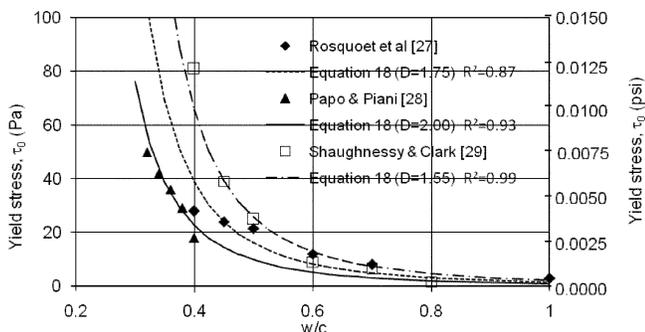
Fig. 7—Curve fitting of published data using Eq. (18).
