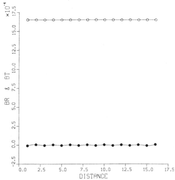
Fig. 7. Radial and circumferential components of flux density on the outer surface of the pipe, for a defect free situation (2D geometry).
