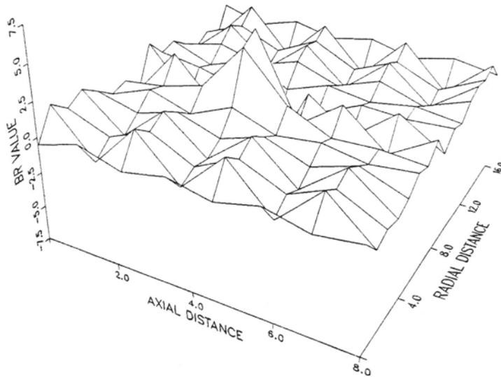
Fig. 9 Leakage field profile due to a three dimensional rectangular slot on the outer surface of pipe wall, showing the error introduced by invalid boundary conditions.
