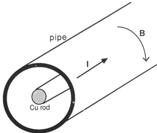
Fig. 2. A generic geometry used for modeling flux leakage method of pipeline inspection.
