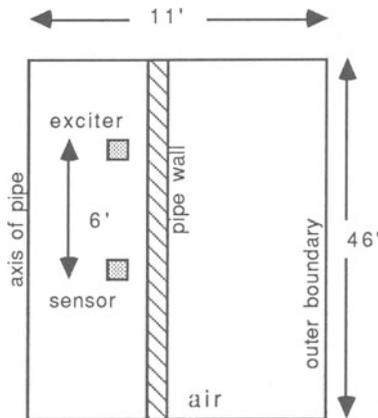
Fig. 3. Typical dimensions encountered in the remote field eddy current inspection of pipelines.
