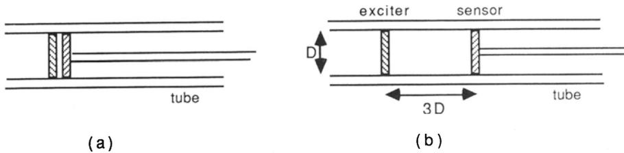
Fig. 1. The geometry of (a) differential eddy current probe (b) remote field eddy current probe.
