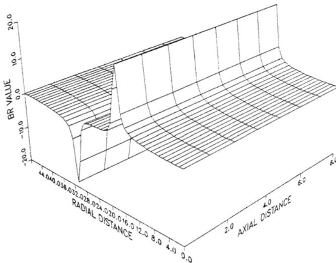
Fig. 8. Leakage field profile for an infinitely long defect (2D geometry) showing validity of the boundary condition in Fig. 6.
