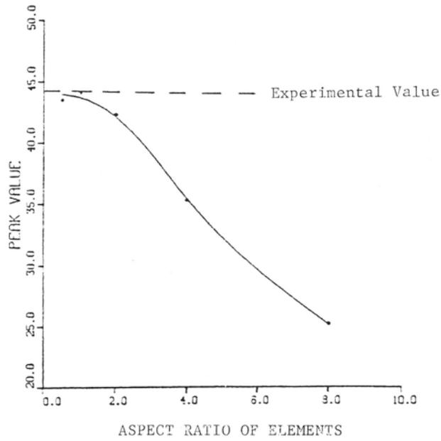
Fig. 4. Variations of the peak amplitude of the flux leakage defect signals with aspect ratio of the elements in the scanning region.
