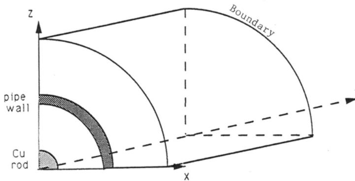
Fig. 5. One quadrant of the geometry in Fig. 2, used in 3D finite element model.
