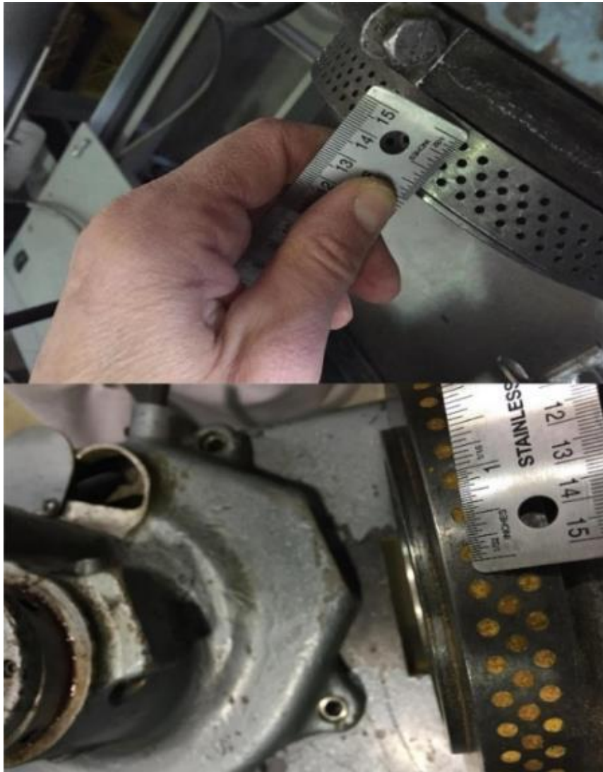
Figure 2. Different dies used in the pelleting process (1/8 in above; 3/16 in below)
