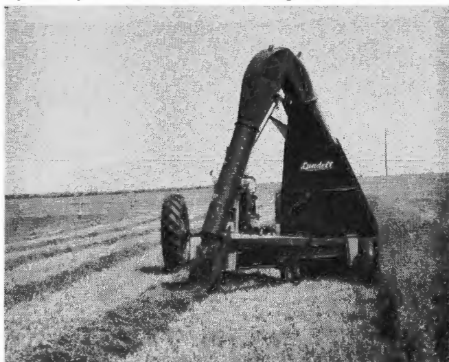
PHOTO 1 (left): A corrugated roller-crimper used in these tests. This machine cracks the stems at uniform intervals. PHOTO 2 (right): A flail-type forage harvester adapted for conditioning hay. The movable downspout can be used as shown to convey the hay from two swaths into a single windrow.
