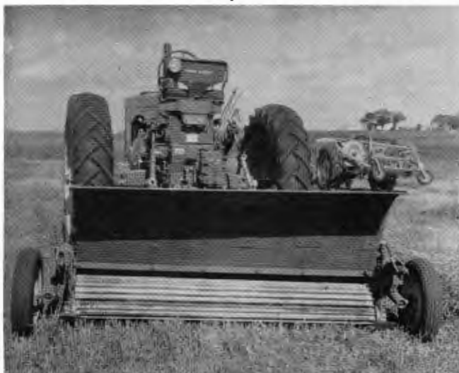
PHOTO 1 (left): A corrugated roller-crimper used in these tests. This machine cracks the stems at uniform intervals. PHOTO 2 (right): A flail-type forage harvester adapted for conditioning hay. The movable downspout can be used as shown to convey the hay from two swaths into a single windrow.
