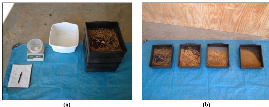
Figure 3. Penn. State Particle Separator on far right (a); four separator sieves and contents (b).
