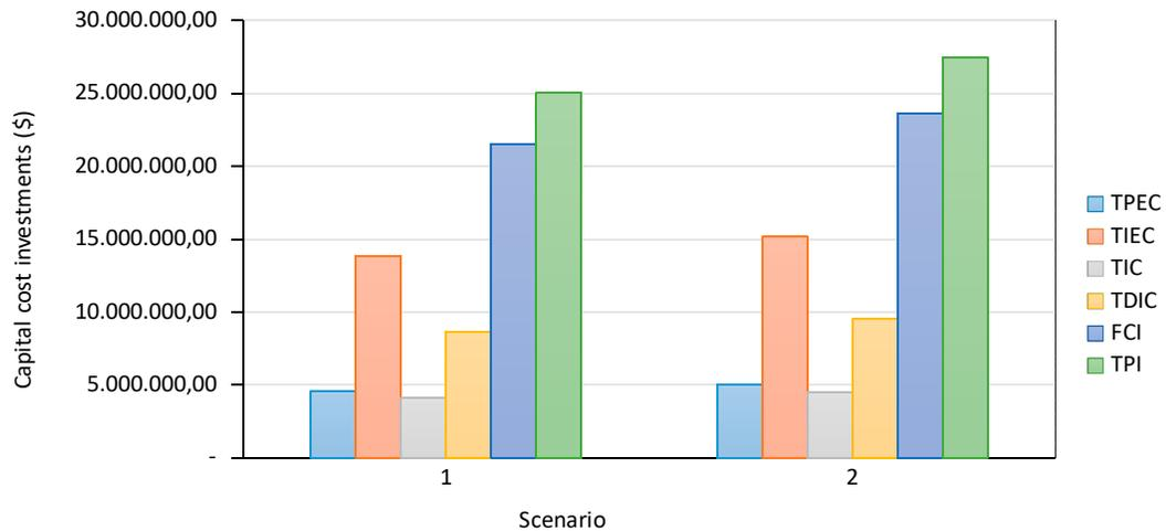
**Figure 3.** Overall fixed capital costs for Scenario I (evaporation process) and Scenario II (flocculation process). TPEC—Total Purchased Equipment Cost; TIEC—Total Installed Equipment Cost; TIC—Total Indirect Cost; TDIC—Total Direct and Indirect Costs; FCI—Fixed Capital Investment; and TPI—Total Project Investment).
