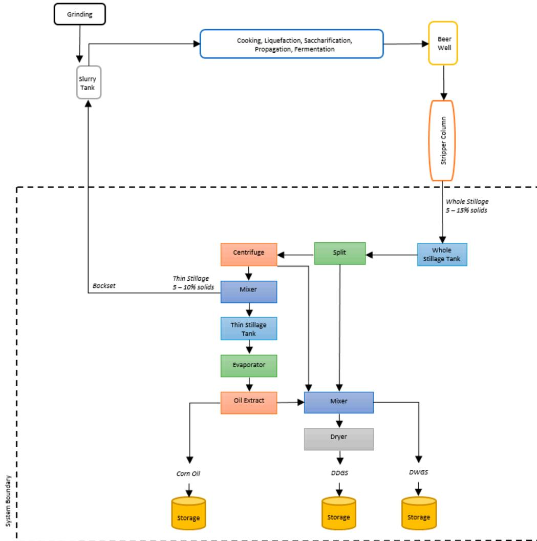
**Figure 1.** Simplified flow diagram of a conventional corn-based ethanol plant flow chart (Scenario I). The system boundary includes tanks, splitter, centrifuge, mixers, dryer, evaporator, and storage systems.
