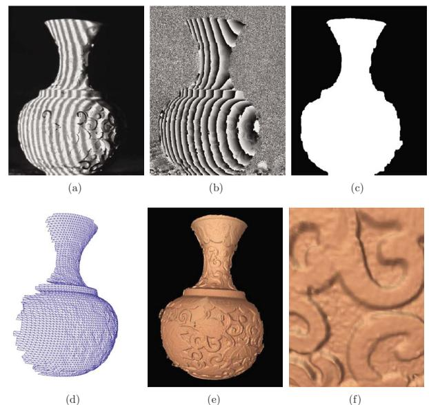
**Fig. 7** Measurement result of the vase (size of the vase is  $\sim 75$  mm in height and 50 mm in width): (a) One final phase-shifted fringe images, (b) the wrapped phase map, (c) the mask used to remove the background, (d) rendered in wireframe mode, (e) rendered in shaded mode, the details of the vase rings are well captured, and (f) zoom-in view of a small region (ring width is  $\sim 1$  mm).
