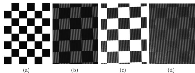
**Fig. 4** Fringe image formation of the checkerboard object: (a) B/W checkerboard, (b) one fringe image with the white squares well illuminated, (c) one fringe image with the black squares well illuminated, and (d) combined fringe image by taking better pixels from (b) and (c).
