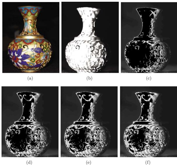
**Fig. 6** Experimental results of the vase: (a) Color photograph of the vase, (b) fringe image for exposure 1, (c) fringe image points usable after exposure 1, (d) fringe image points usable after exposure 2, (e) fringe image points usable after exposure 3, and (f) fringe image points usable after exposure 4.
