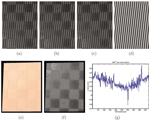
**Fig. 5** Experimental results of a shining object. (a–c) Three fringe images with a phase shift of  $2\pi/3$ , (d) the wrapped phase, (e) 3-D reconstructed result rendered in shaded mode, (f) 3-D result with texture mapping, and (g) cross-section plot of the 320th row.
