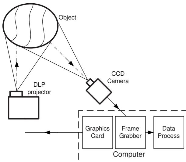
**Fig. 3** System setup.
